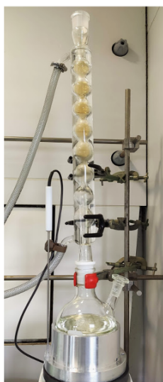
Figure S6. Photograph of the brownish fumes, corresponding to the \text{NO}_x gases released during the reflux heating
