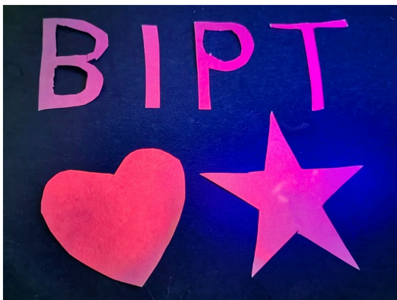
Figure S16. Fluorescent images of CZ-SP and NA-SP as an anti-counterfeiting ink on letters filter paper under UV irradiation for 60 s.
