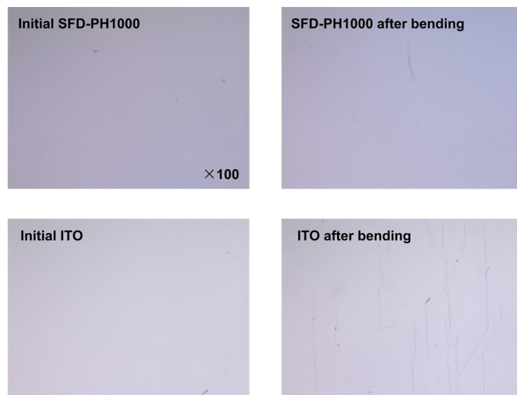
Figure S10. Optical microscope images of PEN/ITO and PEN/SFD-PH1000 before and after 1000 bending cycles.
