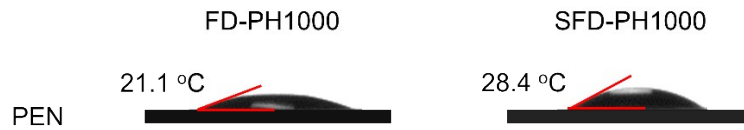
Figure S2. The contact angle of FD-PH1000 and SFD-PH1000 solution on the PEN substrate.
