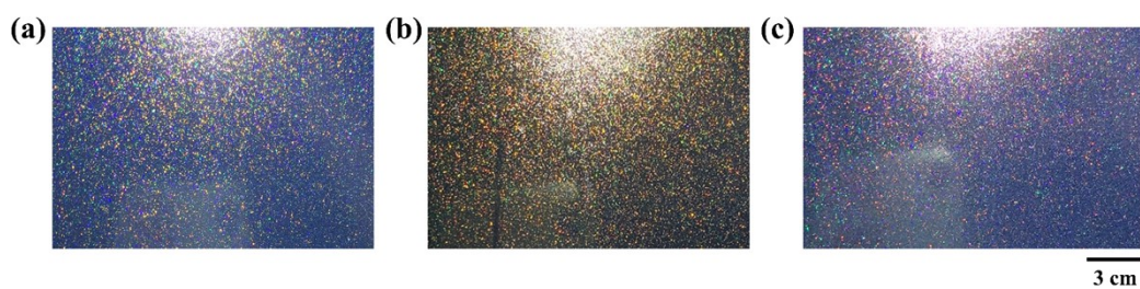
Figure S16 Photonic coatings containing different blending pigments of the same mixing ratios with (a) Y + G + B (1:1:1), (b) R + Y + G (1:1:1) and (c) R + G + B (1:1:1) when weight percentage of pigments is 4 wt%.
