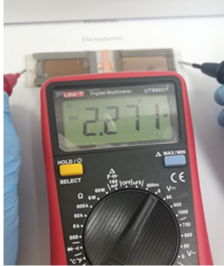
Fig. S24 Measured voltage of two devices in series in the colored state.
