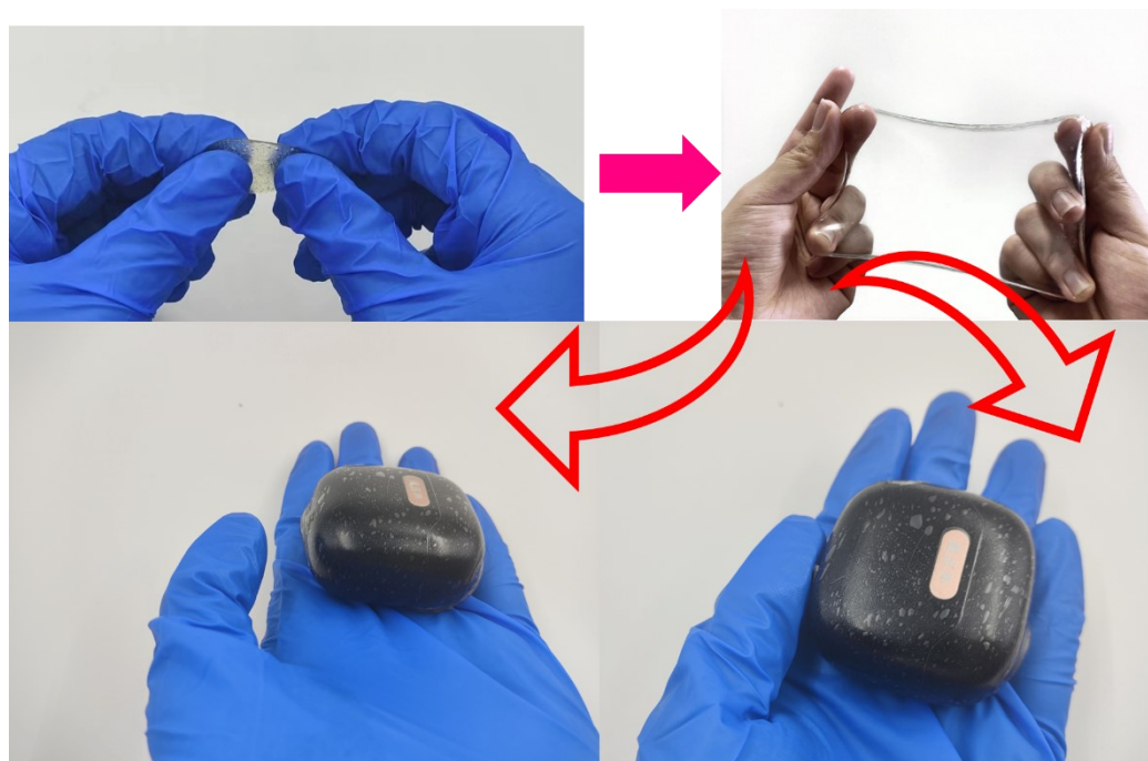
Fig. S7. Tensile ductility and encapsulation of deep eutectic ionic gels
