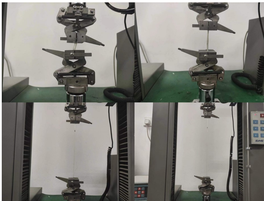
Fig. S9. Testing the tensile properties of deep eutectic ionic gels using an electronic universal tensile machine.
