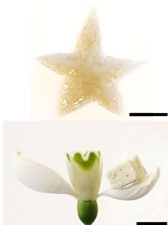
Fig. S2 Photos of the LCPFs with different shapes and low density, scale bar, 1cm.
