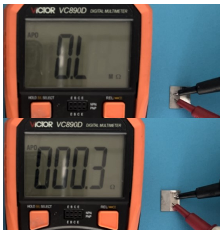
Figure S2. Resistance values of activated and deactivated parts of PPS 2 LM 1.5 film.
