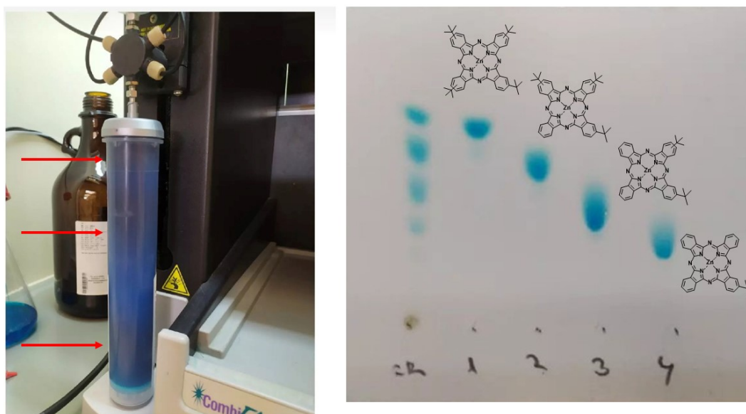
Figure S1. a) ZnPcs 1-4 bands in the chromatography column; b) TLC plate showing the reaction crude vs the different pure fractions of ZnPcs 1-4 in a 5/6 ratio 3:1.
