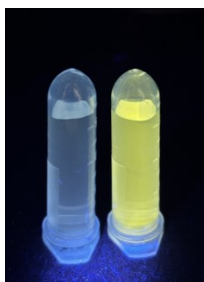
Fig. S9. Fluorescence images of PAA and NBHN aqueous solutions upon the addition of FA under 365 nm UV light.
