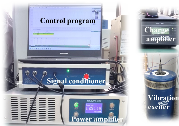
Figure S3. Physical picture of piezoelectric accelerometer testing system.
