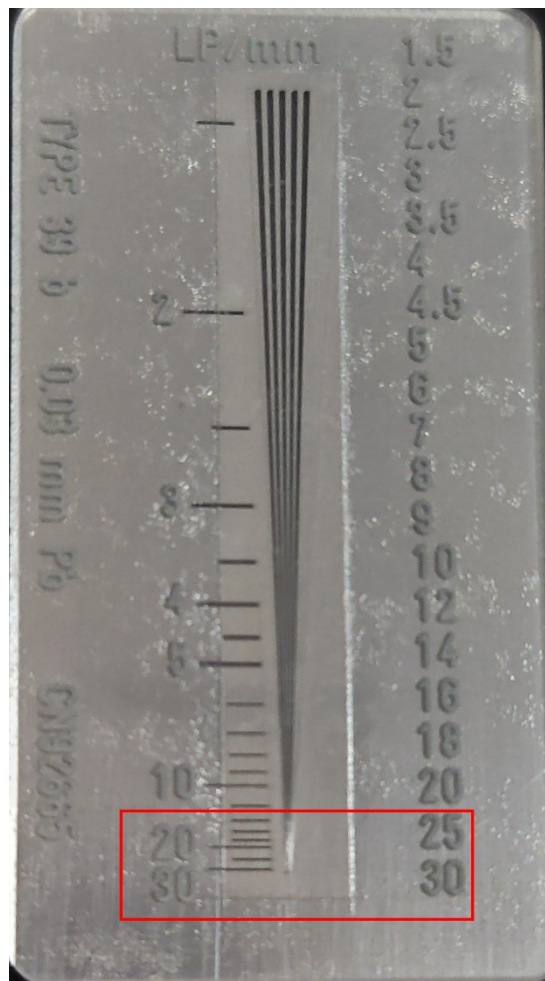
Figure S23. (a) Photographic images of the standard resolution pattern plate. A radiation image resolution card (Type 39b) with 30 lp mm -1 was used for the spatial resolution testing.
