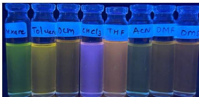
Figure S4. Effect of different solvent polarity on GBY-15 visualized under UV light (365 nm).
