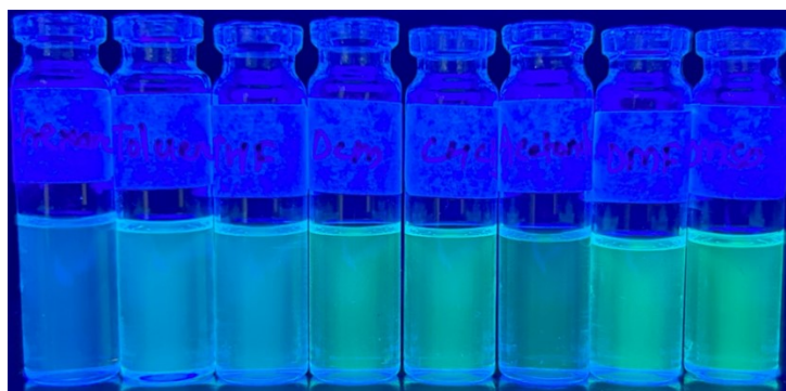
Figure S3. Effect of different solvent polarity on GBY-14 visualized under UV light (365 nm).
