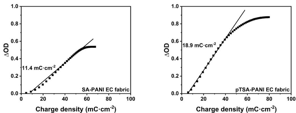
**Figure. S8.** The coloring efficiency of SA-PANI and pTSA-PANI applied to EC fabrics.
