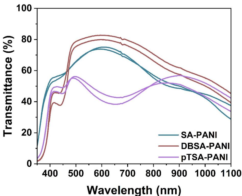
**Figure. S1.** Comparison of spectral transmittance (350 nm - 1100 nm) modulation amplitude of PANI films in reduced state and at 0 V.
