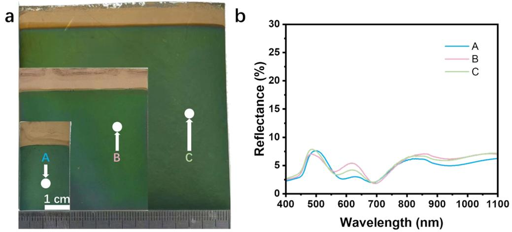
**Figure S10.** (a) Comparison of physical images of EC fabric samples of different sizes and random sampling for spectral measurement. (b) Randomly select points for spectral measurement at 350 nm-1100 nm.
