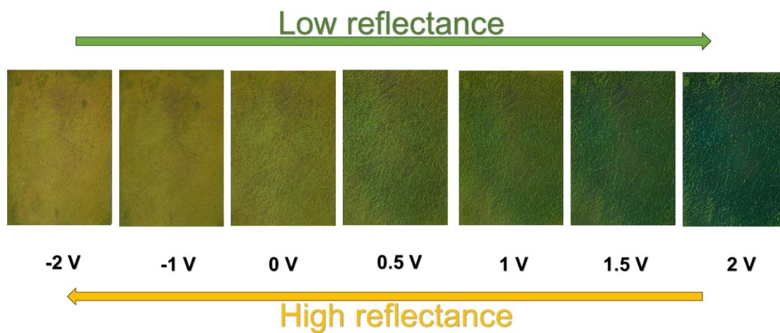
**Figure. S5.** Digital images of EC fabrics: uniform yellow-green transition under an applied voltage of  $\pm 2$  V.
