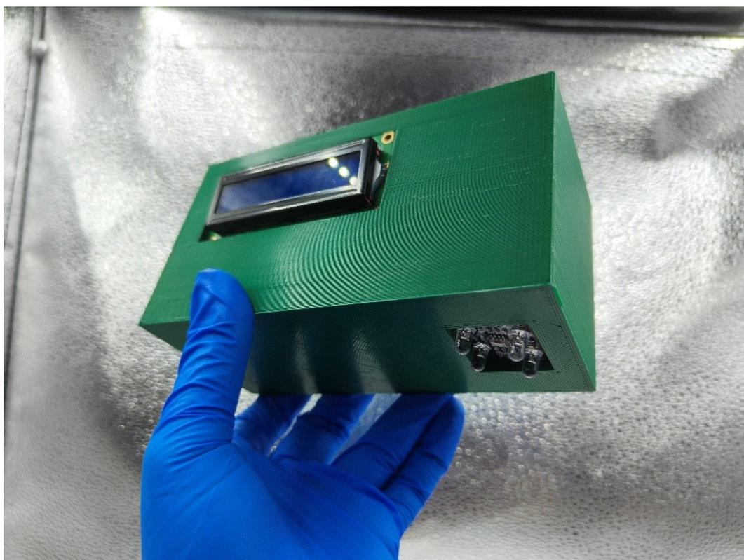
**Figure. S9.** The EAS system integrated into the 3D shell.
