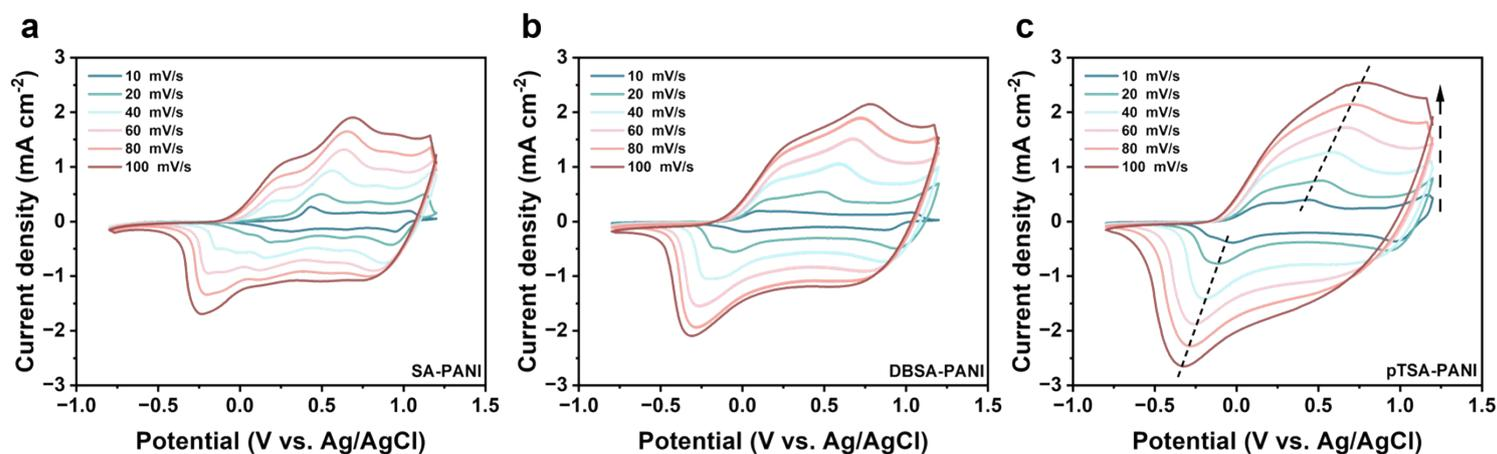
**Figure. S3.** CV curves of three doped PANI at different scanning rates, (a) SA-PANI (b) DBSA-PANI (c) pTSA-PANI.
