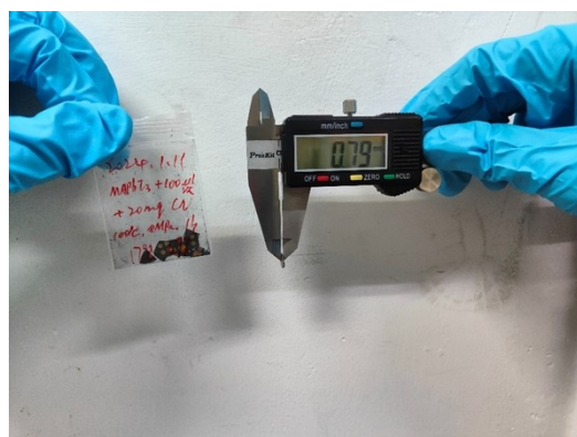
Figure S2. The photo picture during measuring the thickness of the pellet.
