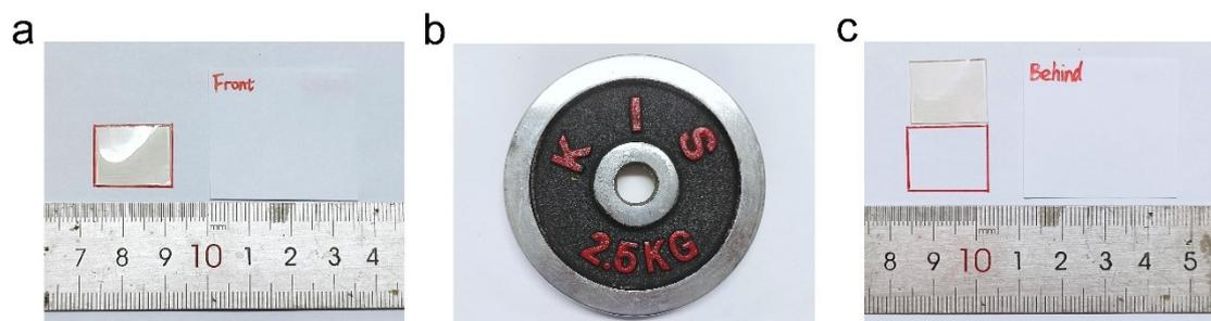
**Fig. S19** The IL retention ability of PU-100IL-10TA at a pressure of 2.5 kg. (a) PU-100IL-10TA with a volume of 18mm x 15mm x 1mm and front side of dry A4 paper measuring 35 × 35mm. (b) PU-100IL-10TA was sandwiched between two sheets of A4 paper and placed under a weight of 2.5kg. (c) After 5 minutes, the weights were removed and the A4 paper underneath the PU-100IL-10TA and the reverse side of the 35 × 35 mm A4 paper (the contact surface with the PU-100IL-10TA) were dry.
