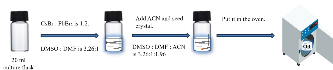
Fig.S1 Schematic diagram of the solution-growth process of CsPbBr 3 single crystal with ACN addition (molar ratios in the figure are indicated).
