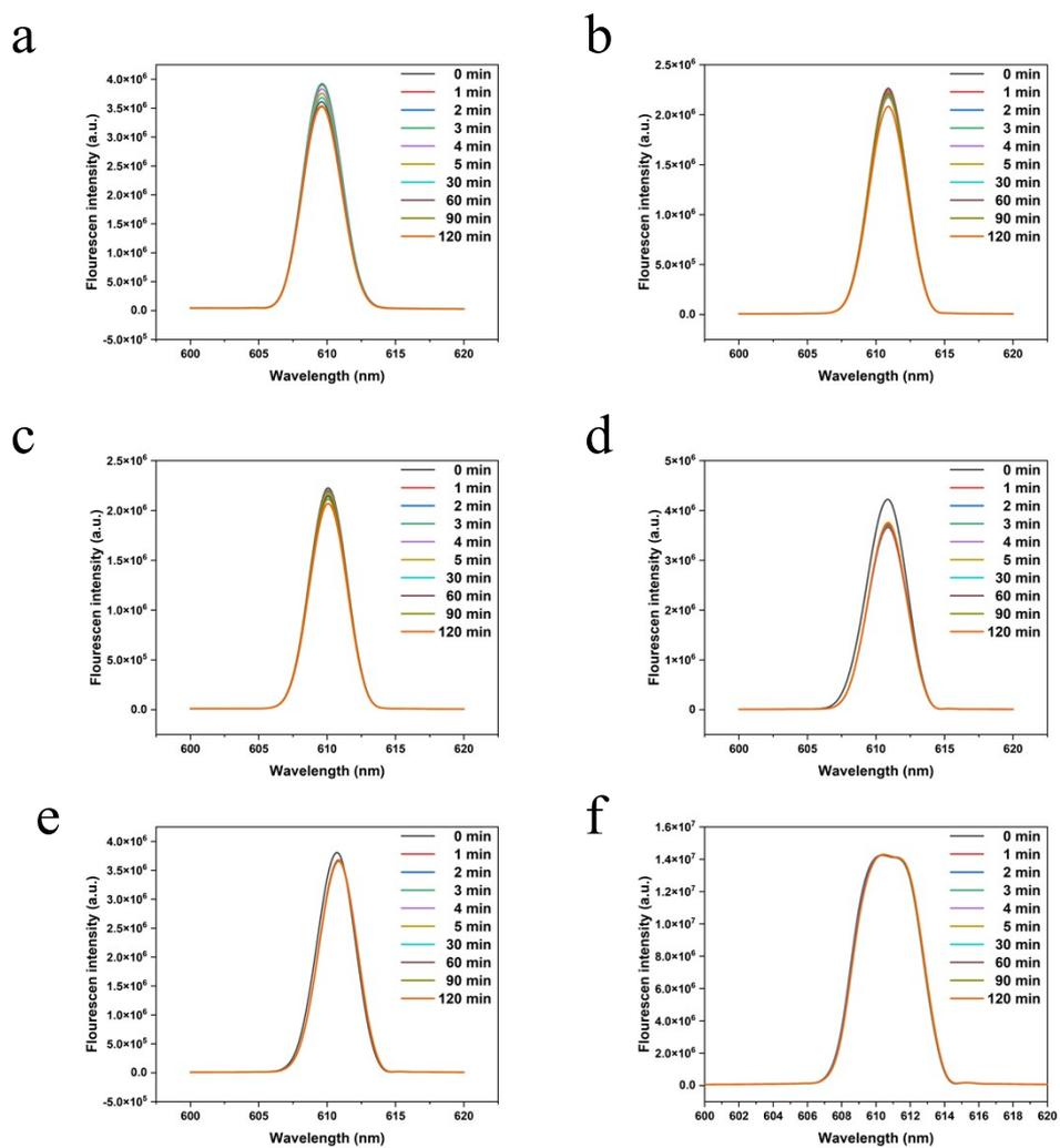
**Fig. S4.** Fluorescence spectrum (a) fluorescence spectrum of PPBD/PEO fiber film in water vapor. (b) fluorescence spectrum of PPBD/PEO fiber film in benzene vapor. (c) fluorescence spectrum of PPBD/PEO fiber film in phenol vapor. (d) fluorescence spectrum of PPBD/PEO fiber film in fragrance vapor. (e) fluorescence spectrum of PPBD/PEO fiber film in urea vapor. (f) fluorescence spectrum of PPBD/PEO fiber film in NaNO<sub>2</sub> vapor.
