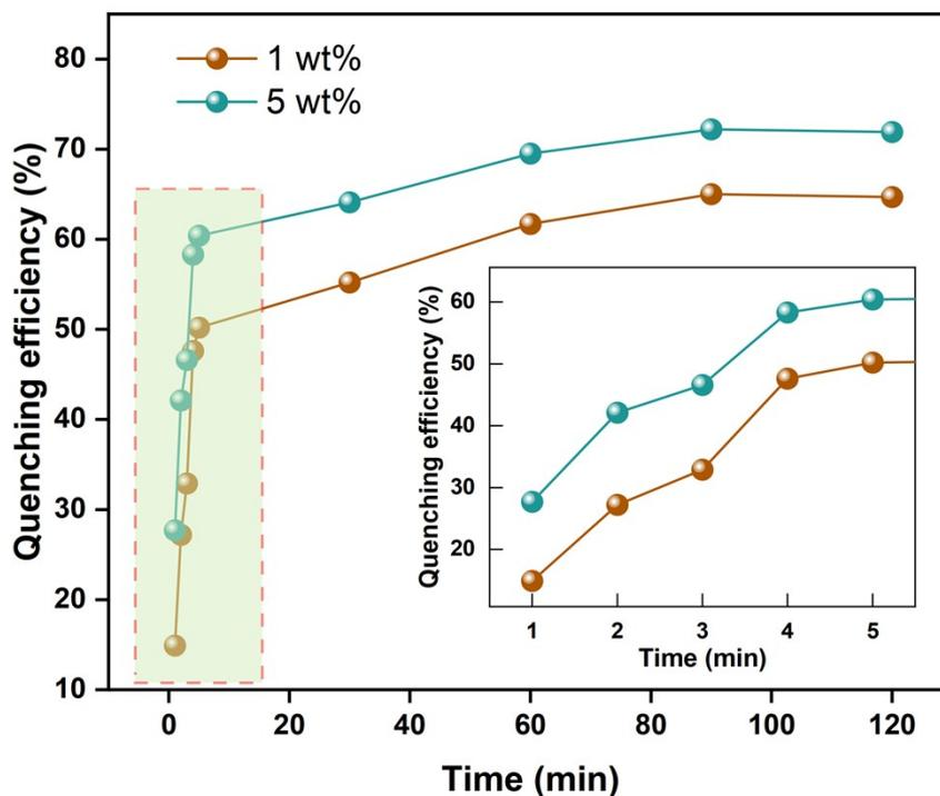
**Fig. S1.** Plot of the fluorescence quenching efficiency versus time of electrospinning membranes doped with different PPBD contents.
