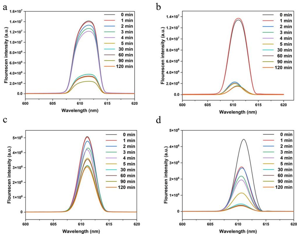
**Fig. S3.** Fluorescence spectrum (a) fluorescence spectrum of PPBD/PEO fiber film in RDX vapor. (b) fluorescence spectrum of PPBD/PEO fiber film in TNT vapor. (c) fluorescence spectrum of PPBD/PEO fiber film in 2,6-dimethylnitrobenzene vapor. (d) fluorescence spectrum of PPBD/PEO fiber film in HMX vapor.
