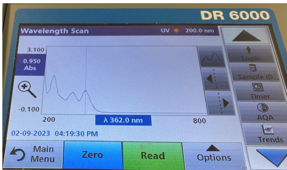
Figure S6. Full scan of 5.5 mg/L \text{Fe}^{3+} in an excess-chloride ethanol solution.
