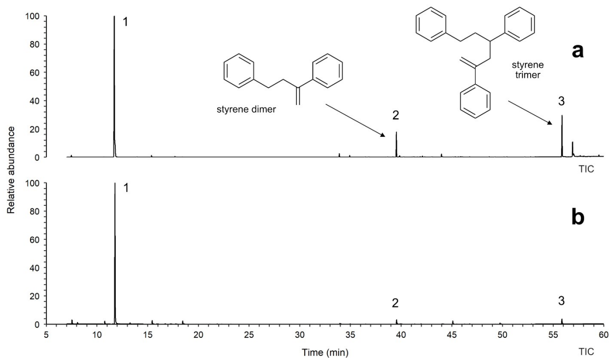
Figure S7. Py-GC/MS chromatograms of PS (a) without thermochemolysis and (b) with thermochemolysis. See Table S8 for peak identification.
