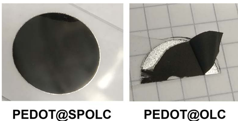
Fig. S3: Differences in electrode manufacturing of PEDOT@SPOLC and PEDOT@OLC , where PEDOT@OLC shows delamination despite the identical electrode manufacturing procedure. Variations also did not lead to improved electrode characteristics.
