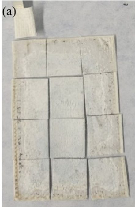
Figure S19: A) Optical image of cycled Cell #1D – anode cell formulation #1 majority Zn vs MnO 2 cathodes (60 wt.% Zn, 26 wt.% CaZn, 10 wt.% Bi 2 O 3 , and 4 wt.% PTFE) b) Table showing the weight and thickness range of the samples.
