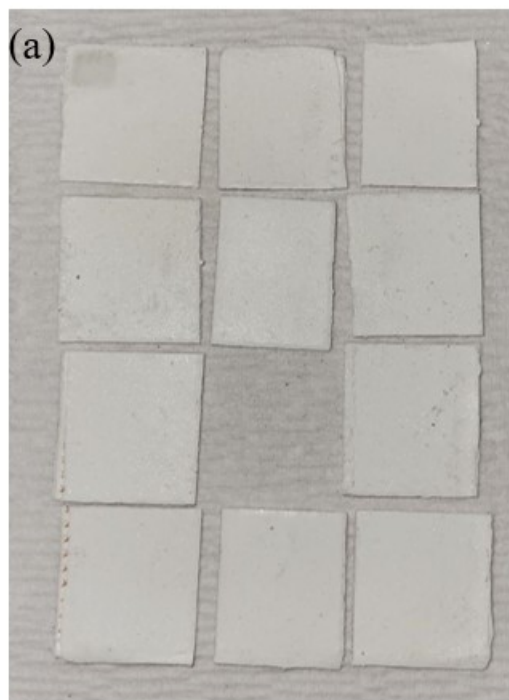
Figure S10: a) Image of freshly rolled and pressed anode cell formulation #3 (86 wt.% CaZn, 10 wt.% Bi 2 O 3 , and 4 wt.% PTFE) dissected for analysis b) Table showing the weight and thickness range of the samples.
