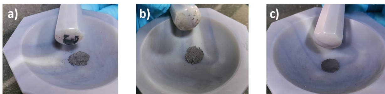
Figure S1: Digital images of Li-GO-EnBoc electrode fabrication with different concentration of binder (a) 10% (b) 20% and (c) 30%.
