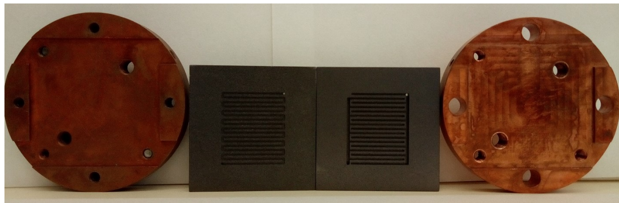
Figure 1S: RFB cell's components: copper plates current collectors and graphite plates with flow channels.
