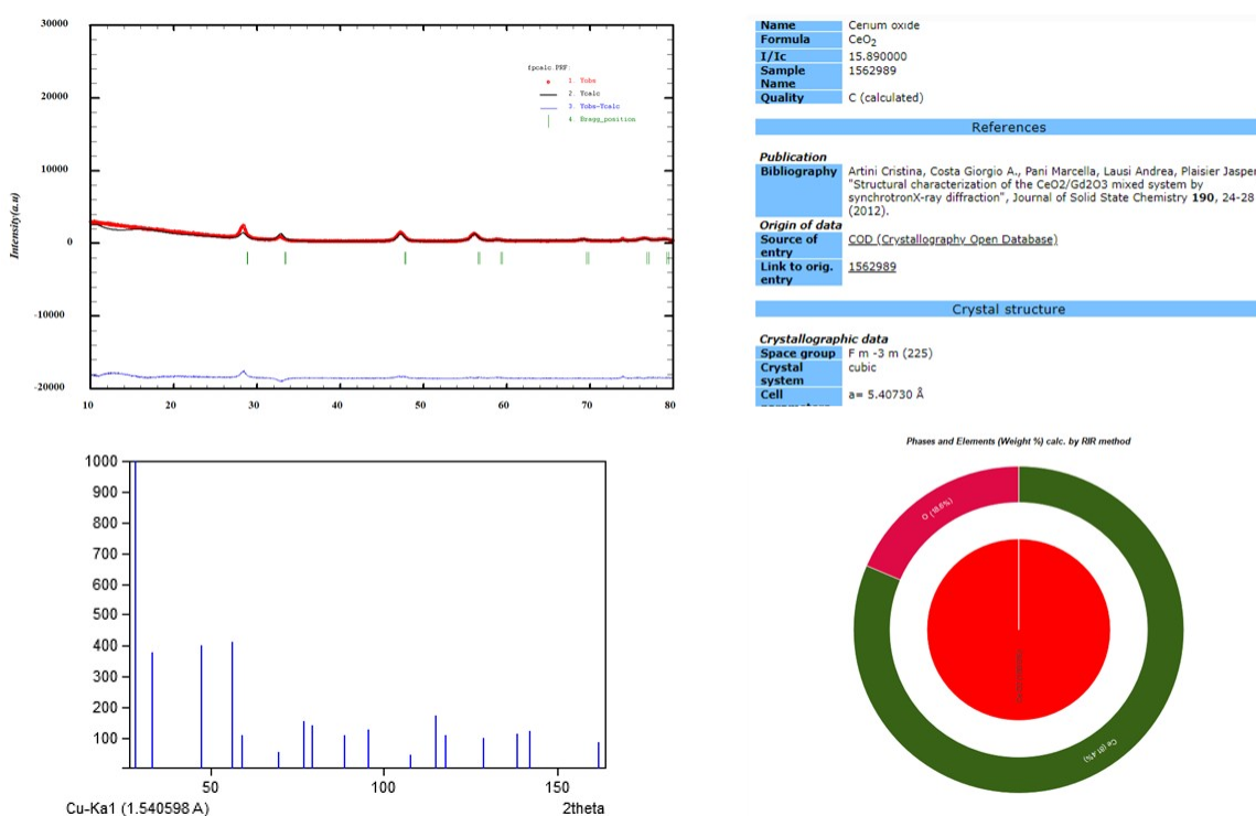
Figure S1. Rietveld analysis of CeO_2 photocatalyst and composition of the CeO_2 photocatalyst
