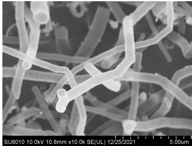
Figure S5 SEM image of NCNT.
