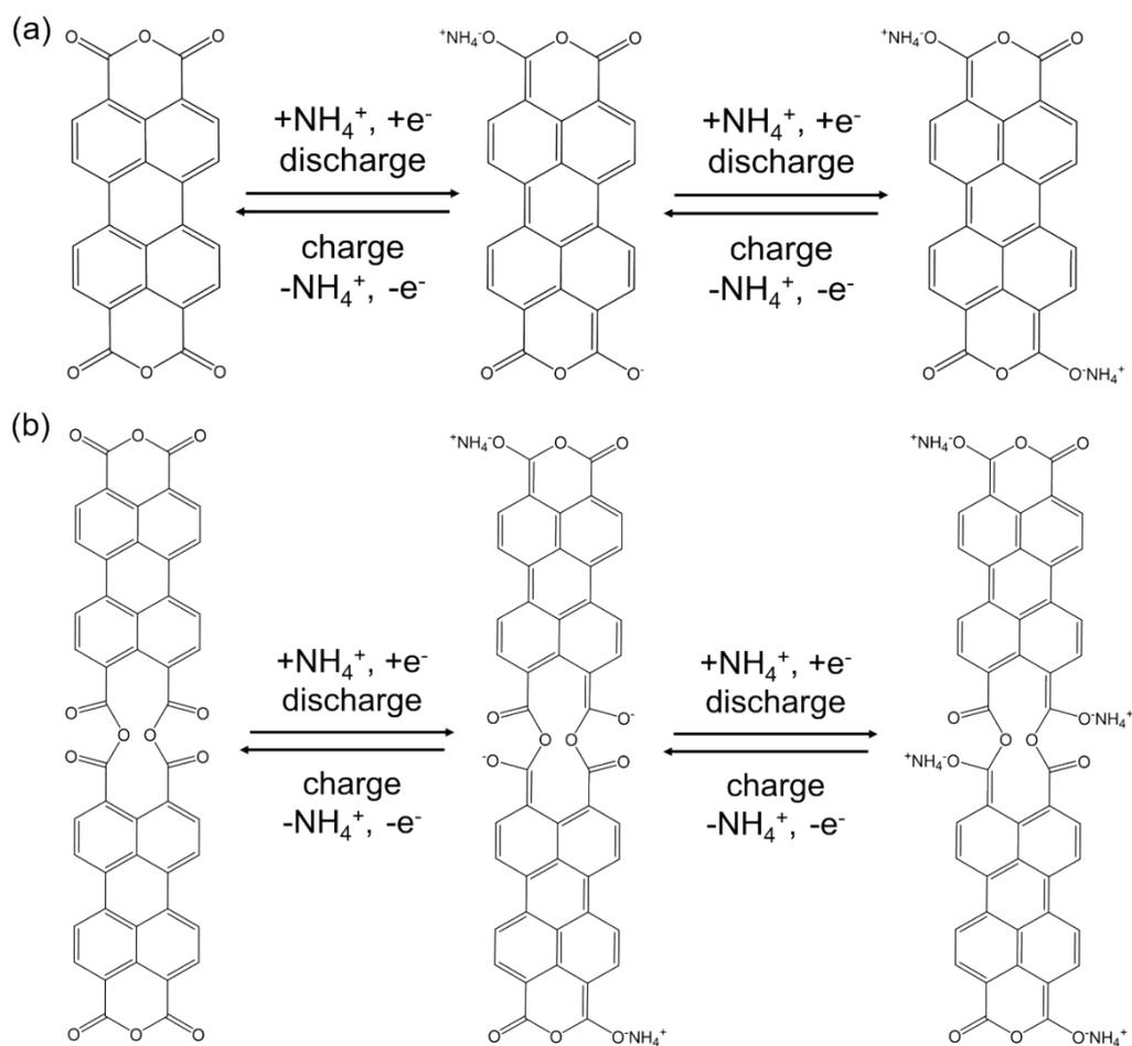
**Fig. S10** Proposed  $\text{NH}_4^+$  incorporation mechanism of (a) PTCDA and (b) P420.
