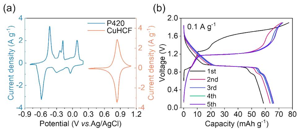
**Fig. S13** (a) CV curves of Cu-HCF cathode and P420 anode at  $2 \text{ mV s}^{-1}$ . (b) GCD profiles of the first five cycles at  $0.1 \text{ A g}^{-1}$ .
