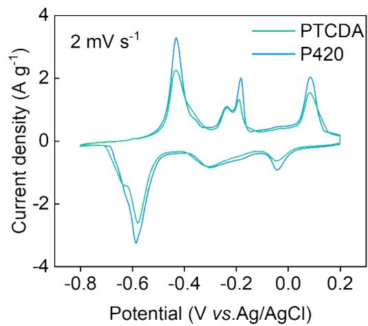
**Fig. S6** CV curves of PTCDA and P420 anodes at 2 mV s<sup>-1</sup>.
