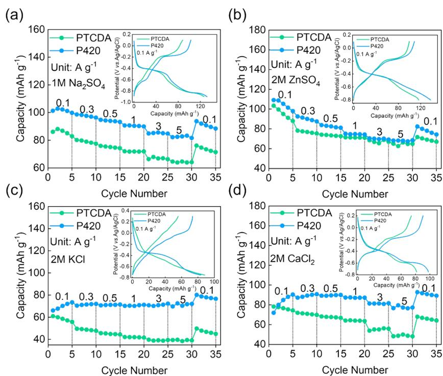
**Fig. S9** Rate capacities and GCD curves of different metal-ion electrolytes at pristine PTCDA and P420. (a) 1M Na<sub>2</sub>SO<sub>4</sub>. (b) 2M ZnSO<sub>4</sub>. (c) 2M KCl. (d) 2M CaCl<sub>2</sub>.
