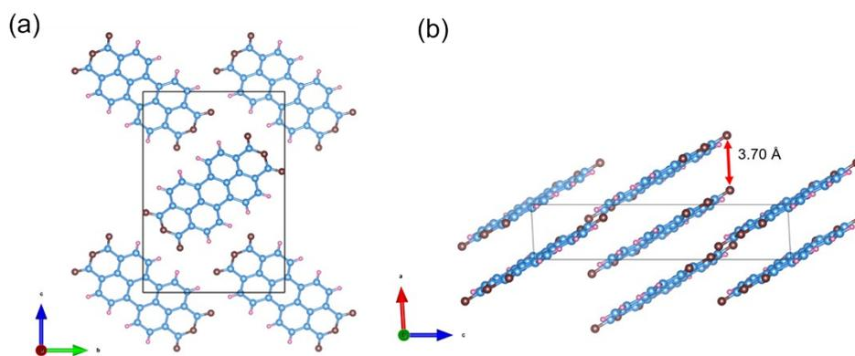
**Fig. S4** Crystalline structure of  $\alpha$ -PTCDA. The blue, pink, and brown spheres represent C, H, and O atoms, respectively.
