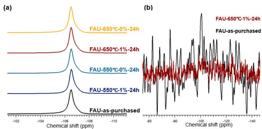
**Figure S3**  $^{29}\text{Si}$  single-pulse MAS NMR (a) and CP MAS NMR (b) spectra of FAU-as-purchased and selected treated samples.
