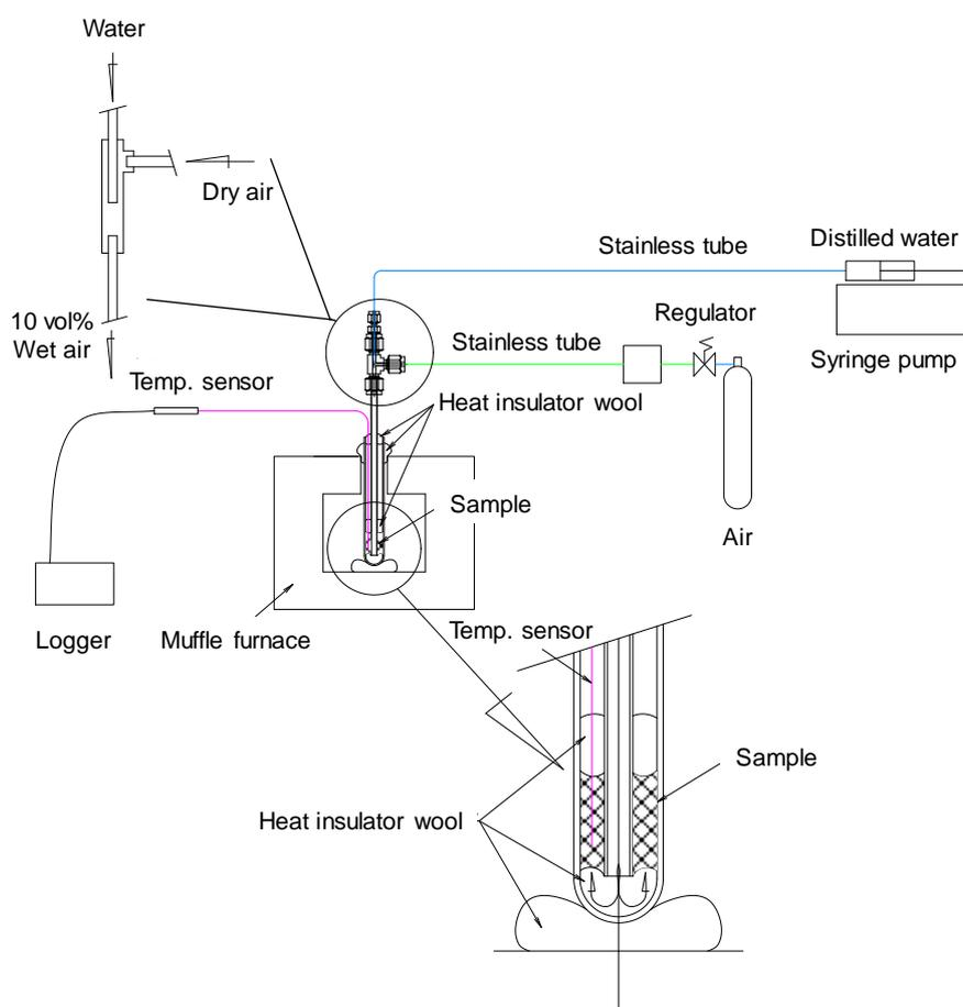
**Figure S1** The custom-built apparatus for the steam treatment.<sup>[5]</sup>
