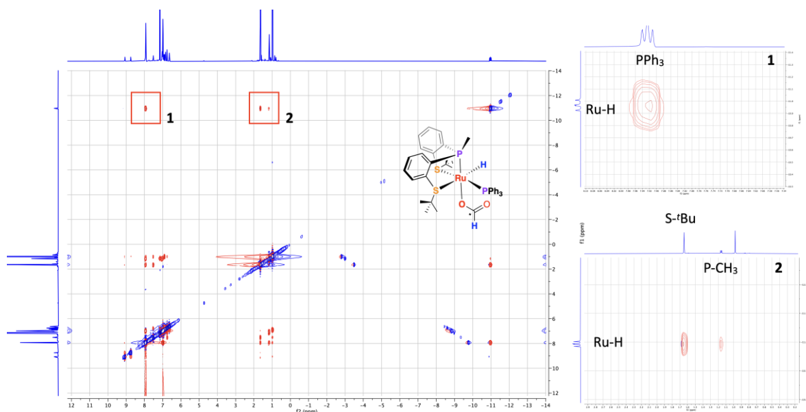
Figure S22. ^1\text{H} NOESY NMR of ^{13}\text{CO}_2 derived 1-HCO 2 in \text{C}_6\text{D}_6 (left) and an inset (right) showing an NOE correlation between the hydride ligand and the aromatic protons from PPh 3 ( 1 ) and P(CH 3 ) ( 2 ).
