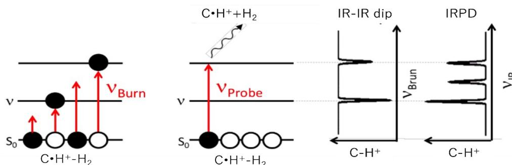
Figure S2: Schematic representation of the IR-IR double resonant spectroscopy technique.
