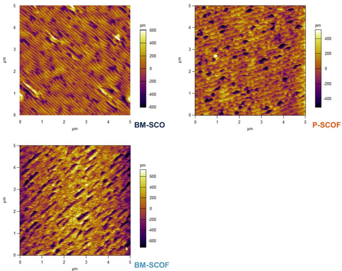
**Figure S1.** AFM surface topography of BM-SCO, P-SCOF, and BM-SCOF thin films.
