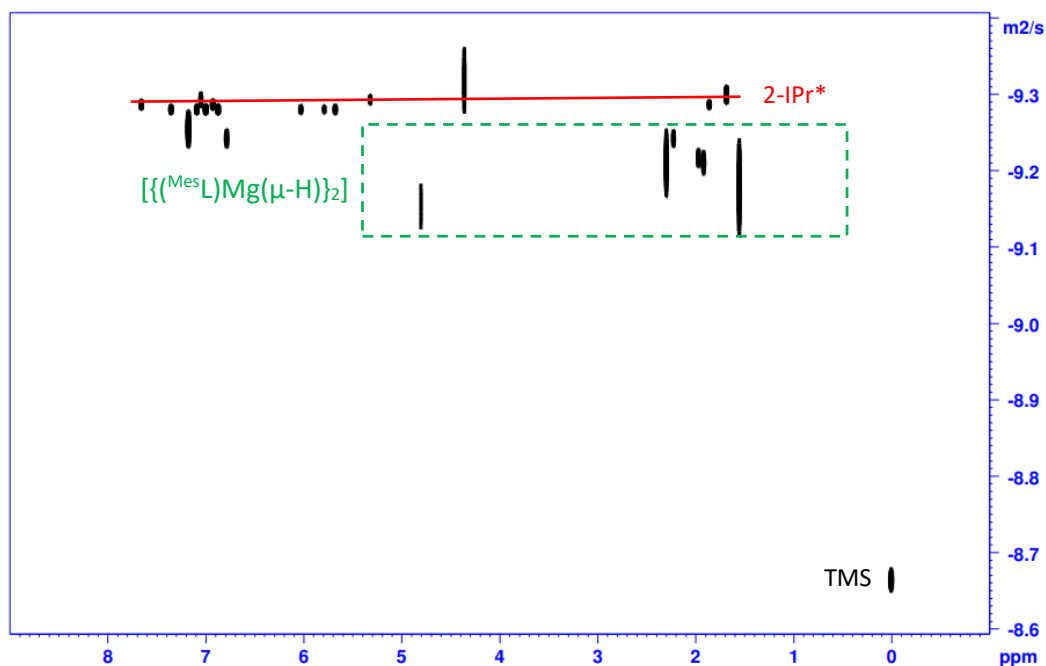
Figure S4. ^1\text{H} DOSY NMR spectrum of 2-IPr* in \text{C}_6\text{D}_6 with TMS as standard in \text{C}_6\text{D}_6 .
