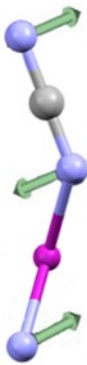
Figure S2. Calculated eigenvectors of selected phonon modes in 30.9 meV at the gamma point.
