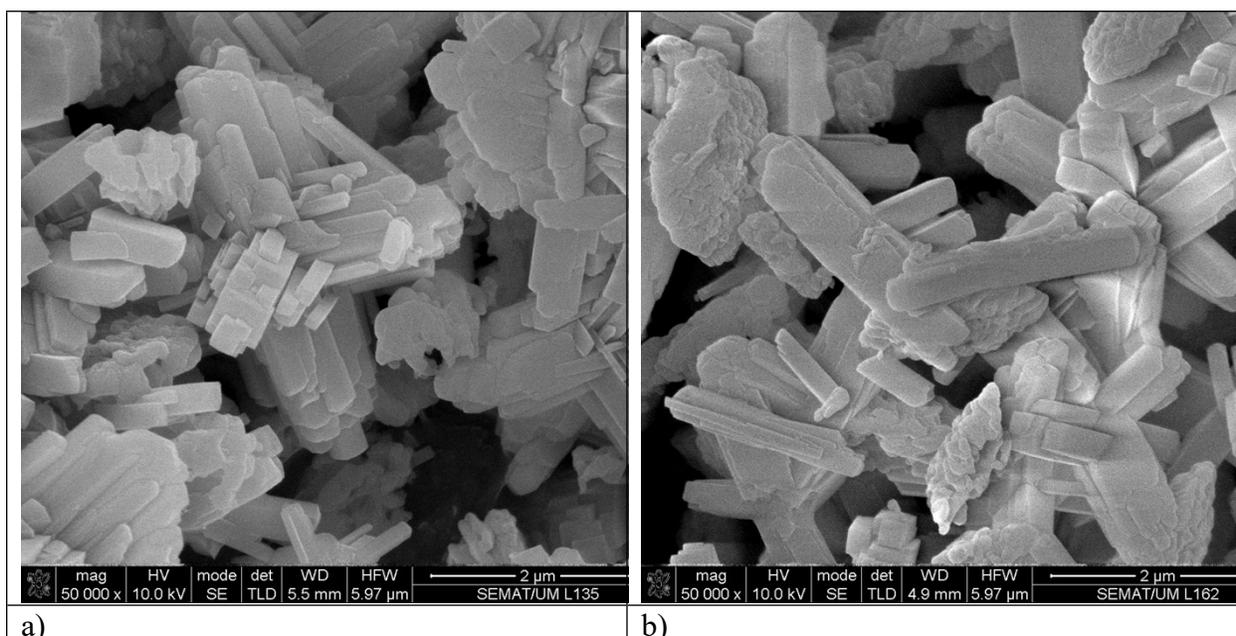
Figure S7. SEM of **MER** zeolite obtained at (a) 150 °C and (b) 160 °C in the system: 0.5 g FAU-1 g KOH - 4.5 g H<sub>2</sub>O for 15 min.
