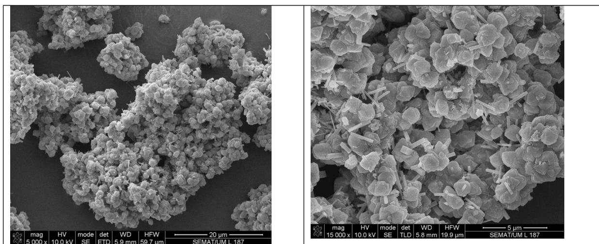
Figure S8. Different magnification images of **LTJ** zeolite obtained at 160 °C for 15 min in the system: 0.15 g FAU – 1 g KOH – 4.5 g H<sub>2</sub>O.
