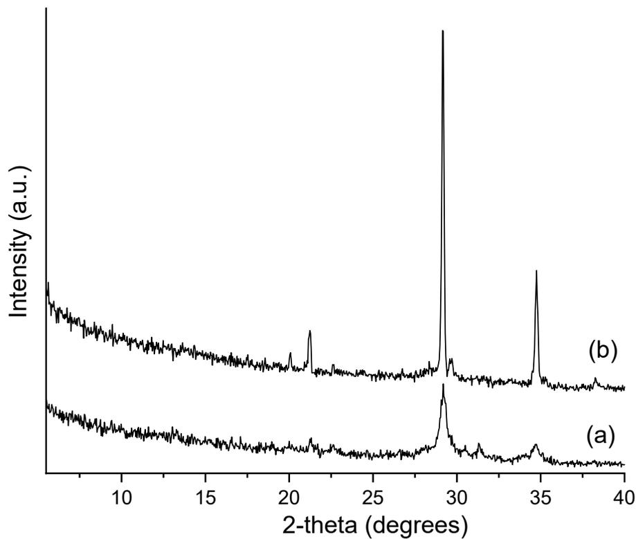
Figure S1. Powder XRD patterns show the formation of  $\text{KAISiO}_4$  at (a) 80 °C for 185 min and (b) at 160 °C for 15 min in the system: 0.5 g FAU – 4.47 g KOH – 3.9 g  $\text{H}_2\text{O}$ .
