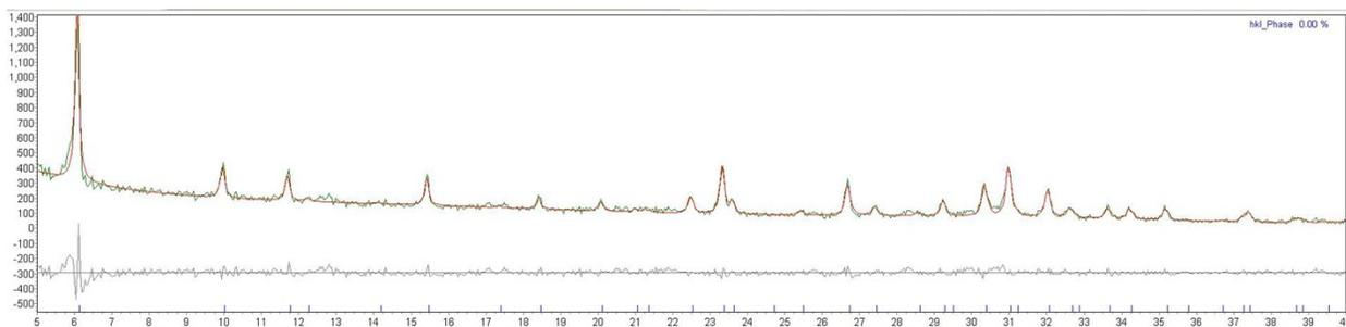
Figure S2. Le Bail fit of FAU zeolite obtained after desilication at 130 °C for 15 min.
