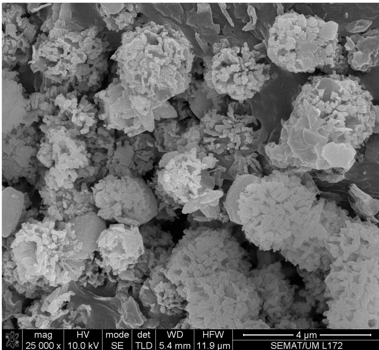
Figure S5. SEM image of partially dissolved FAU zeolite obtained at 130 °C for 15 min.
