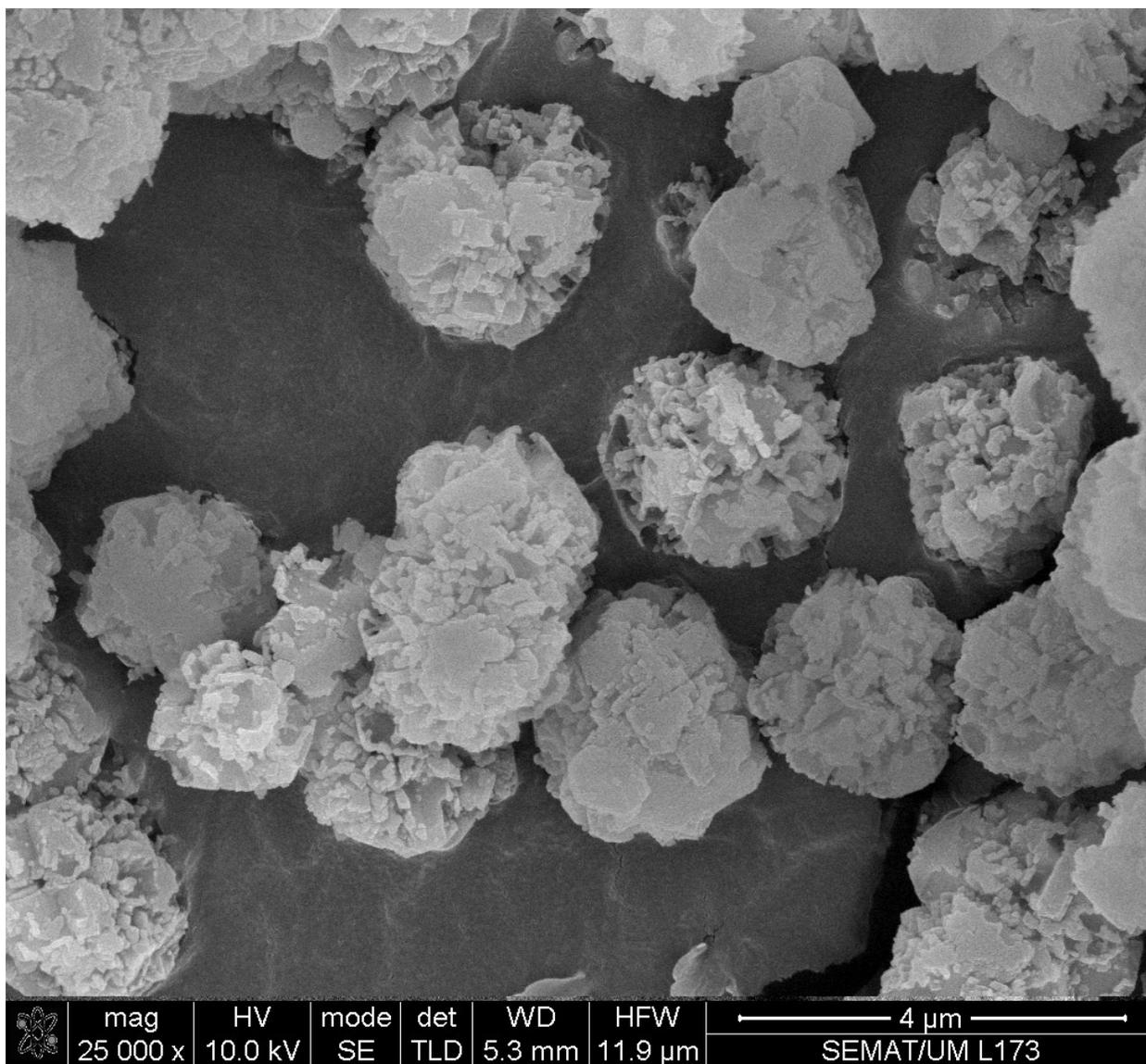
Figure S6. SEM image of partially dissolved FAU zeolite obtained at 140 °C for 15 min.
