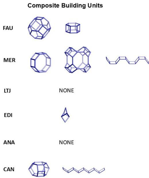
Figure S4. Comparison between the composite building units of the parent **FAU** zeolite the daughter zeolites.
