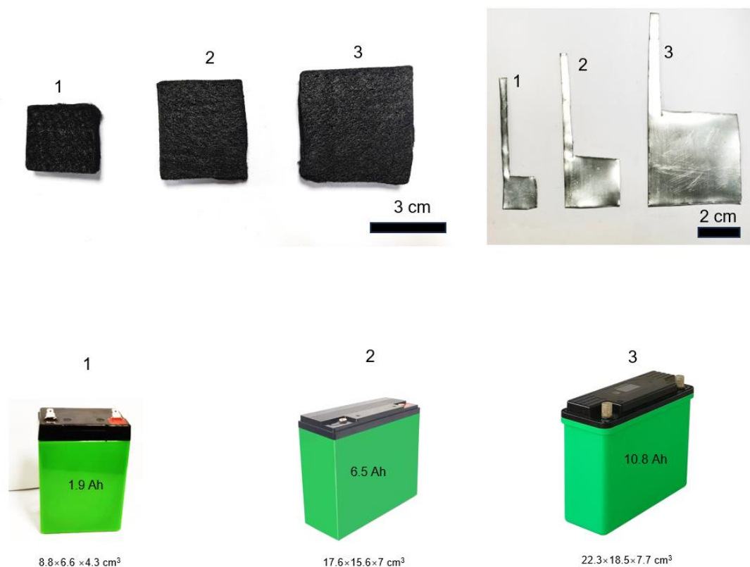
Fig. S19 Photographs of the assembled DPZIB for Ah-level cell tests. Upper row: the carbon film and Zn plates of different sizes used in the corresponding cells in the bottom row.
