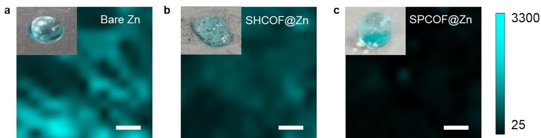
**Figure S15.** 2D Raman mapping on the surfaces of bare Zn (a), SHCOF@Zn (b) and SPCOF@Zn(c) after immersion in electrolyte for 7 days. insets show images of the interfaces between various electrodes and electrolyte, with the electrolyte visualized using methyl blue staining, scale bar: 10 um.
