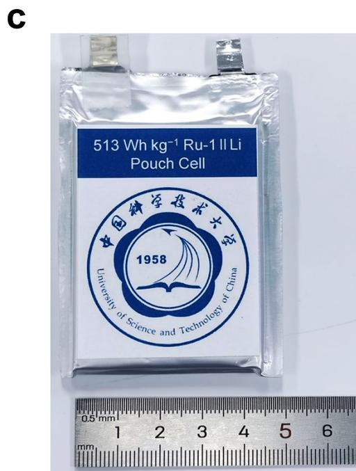
**Figure S21 (a)** The screenshot of the Ru-1||Li test results (discharge capacity, discharge energy, and discharge median voltage) captured from Neware battery test software. The optical images of **(b)** the pouch cell weight and **(c)** the pouch cell size measurements.
