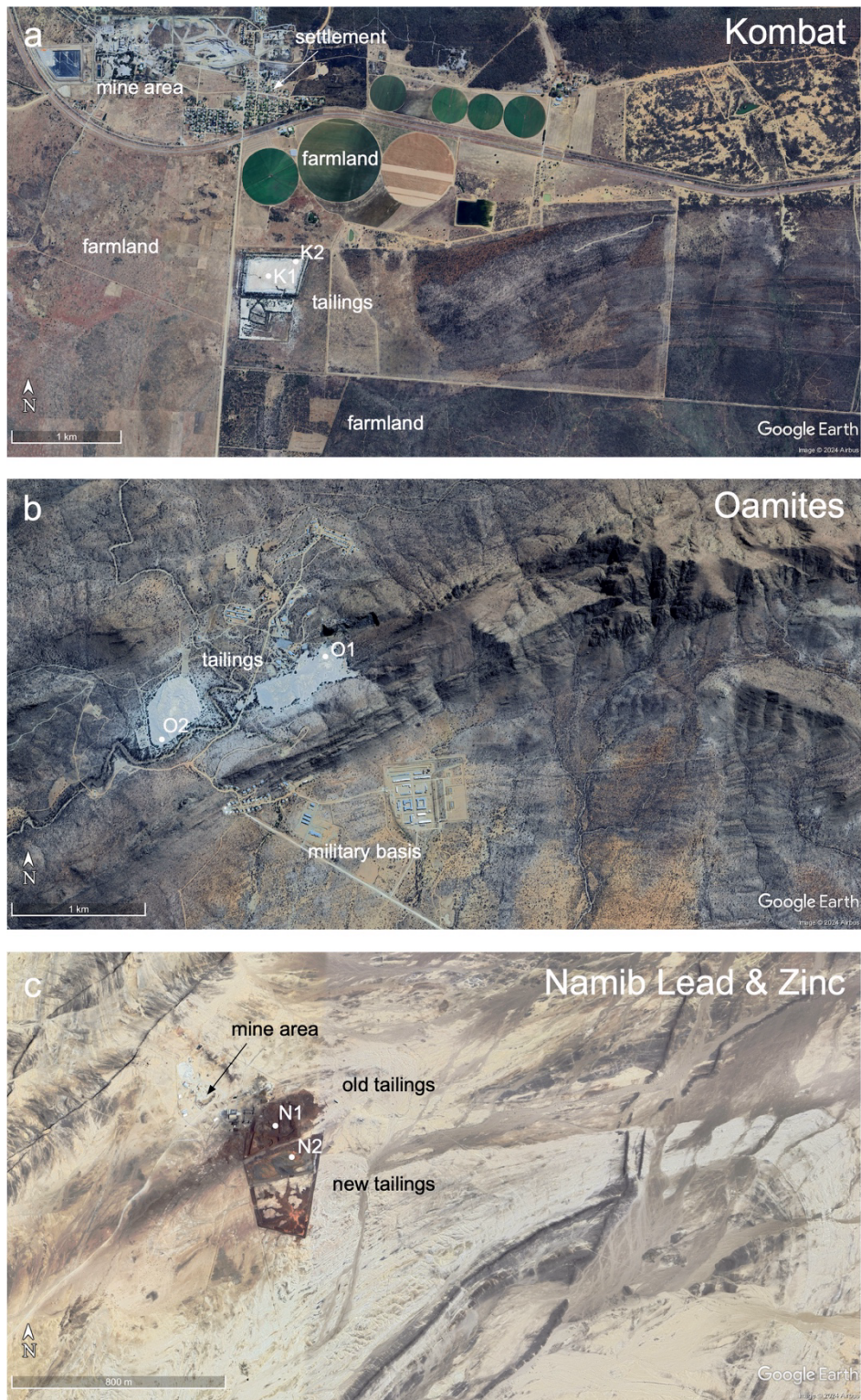
Figure S2. Satellite photographs (based on Google Earth™) of the study sites: Kombat (a), Oamites (b), and Namib Lead & Zinc (c) with indication of the tailings disposal sites, mine areas, settlements, and farmland.
