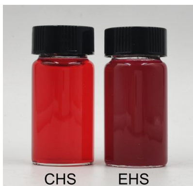
Figure S7 The dyes distributed with time conventional H 2 O system (CHS) and EtOH-H 2 O solvent system (EHS).
