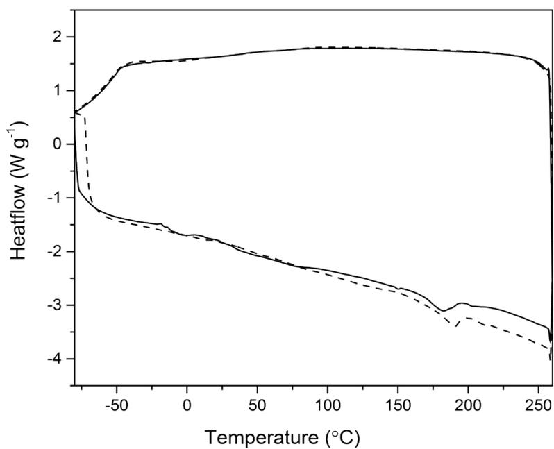
**Figure S9.** DSC traces of **PU<sub>L</sub>-AM-1**. Bold solid line: first heating/cooling cycle, dashed line: second heating/cooling cycle.
