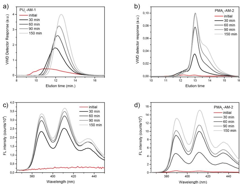
**Figure S5.** SEC traces (VWD) of (a) **PU<sub>L</sub>-AM-1** (347 nm) and (b) **PMA<sub>L</sub>-AM-2** (254 nm) measured at time zero and after being exposed to 30, 60, 90, and 150 min of ultrasonication. 347 nm was selected for **PU<sub>L</sub>-AM-1** due to the polyurethane itself absorbing strongly at 254 nm. Fluorescence spectra of (c) **PU<sub>L</sub>-AM-1** and (d) **PMA<sub>L</sub>-AM-2** measured at time zero and after being exposed to 30, 60, 90 and 150 min of ultrasonication.
