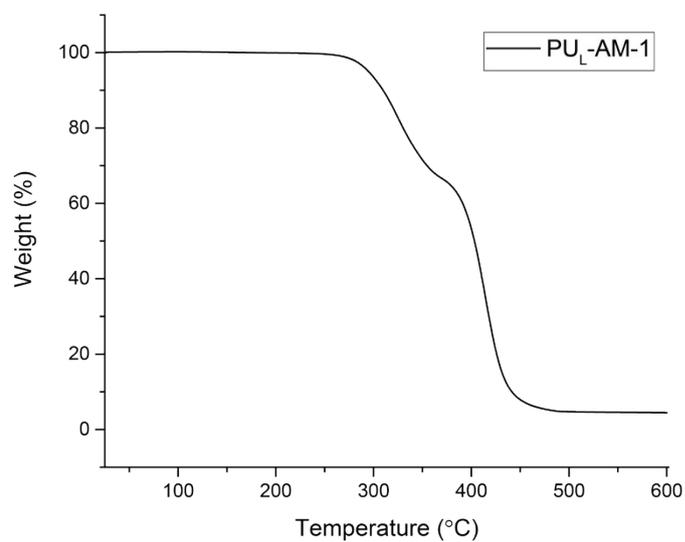
Figure S13. TGA curve of PU<sub>L</sub>-AM-1.
