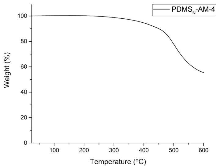
**Figure S16.** TGA curve of PDMS<sub>N</sub>-AM-4.
