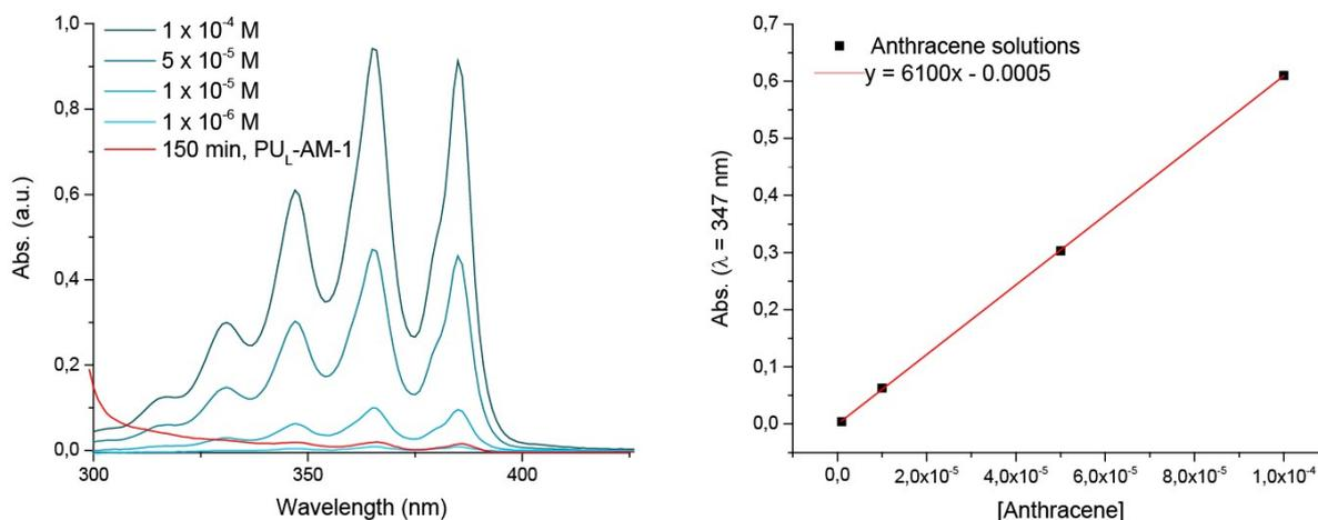
**Figure S7.** (left) UV-Vis spectra of anthracene solutions (THF) of known concentrations and PU<sub>L</sub>-AM-1 after 150 minutes of effective sonication time (red curve). (right) Plot of anthracene absorbance at 347 nm in THF vs anthracene concentration to determine molar extinction coefficient.
