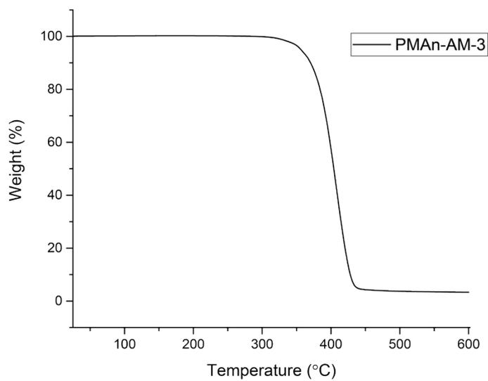
Figure S15. TGA curve of PMA<sub>N</sub>-AM-3.
