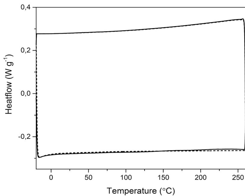
Figure S12. DSC traces of PDMS<sub>N</sub>-AM-4. Bold solid line: first heating/cooling cycle, dashed line: second heating cycle.
