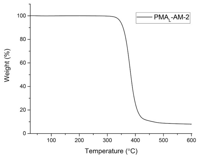
Figure S14. TGA curve of PMA<sub>L</sub>-AM-2.
