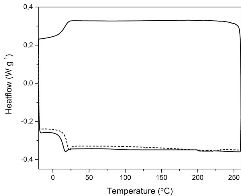
**Figure S10.** DSC traces of PMA<sub>L</sub>-AM-2. Bold solid line: first heating/cooling cycle, dashed line: second heating cycle.
