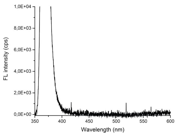
**Figure S19.** Fluorescence spectrum of a PDMS<sub>N</sub>-AM-4 film after elongation to failure.
