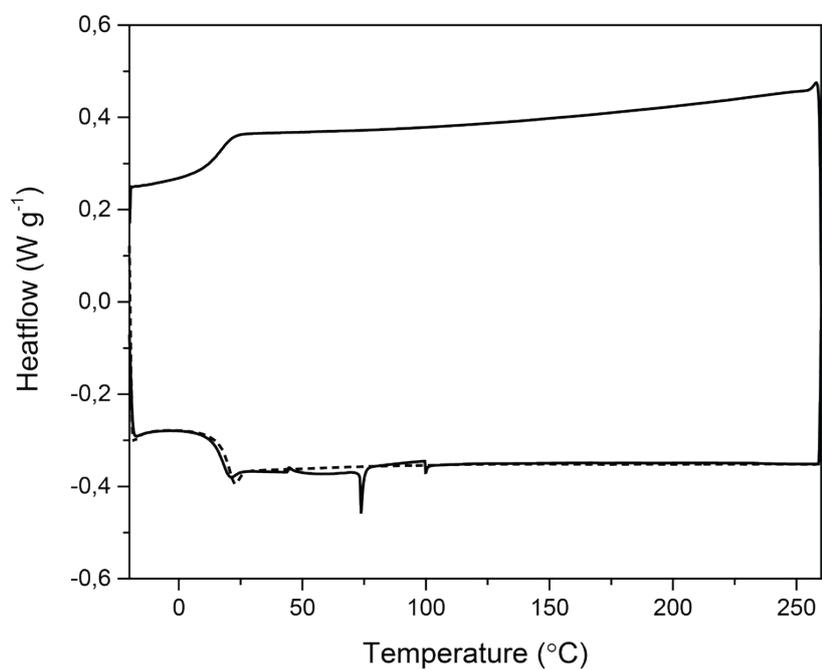
**Figure S11.** DSC traces of PMA<sub>N</sub>-AM-3. Bold solid line: first heating/cooling cycle, dashed line: second heating cycle.
