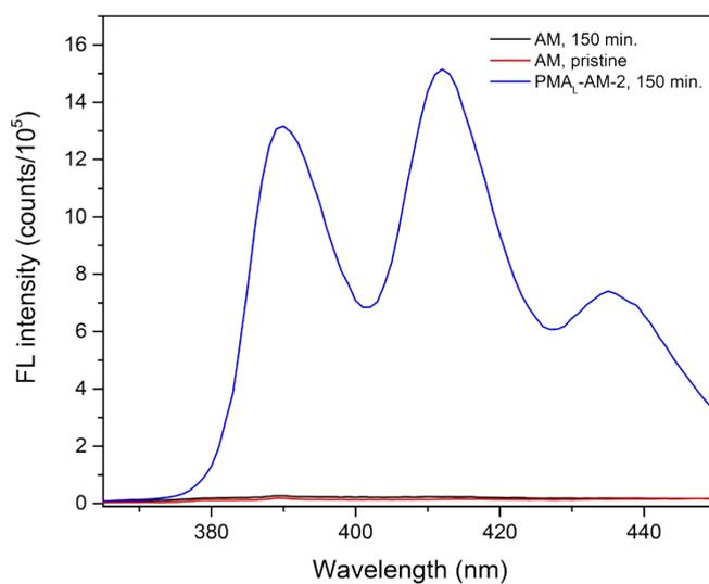
**Figure S6.** Fluorescence spectra of a small molecule **AM-4** solution in THF (15 μg/mL) before and after being exposed to 150 minutes of effective sonication time, compared to the fluorescence spectrum of **PMA<sub>L</sub>-AM-2** after 150 minutes of effective sonication time.
