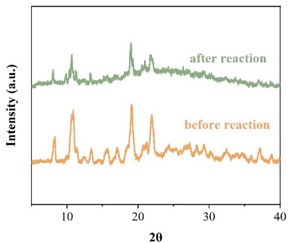
Figure S12. PXRD of HNU-94-120 before and after photocatalytic reaction.
