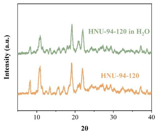
Figure S2. PXRD of HNU-94-120 after 48 h immersion in H<sub>2</sub>O.
