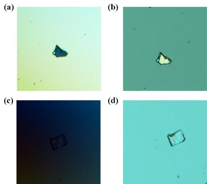
**Figure S7.** (a) Original single crystal polarized optical microscope image and (b) A single crystal corresponding to complete extinction for  $\text{Hg}_3\text{O}_2(\text{NO}_3)_2 \cdot \text{H}_2\text{O}$ ; (c) Original single crystal polarized optical microscope image and (d) A single crystal corresponding to complete extinction for  $(\text{CH}_5\text{N}_3\text{S})_2\text{Hg}(\text{NO}_3)_2$ .
