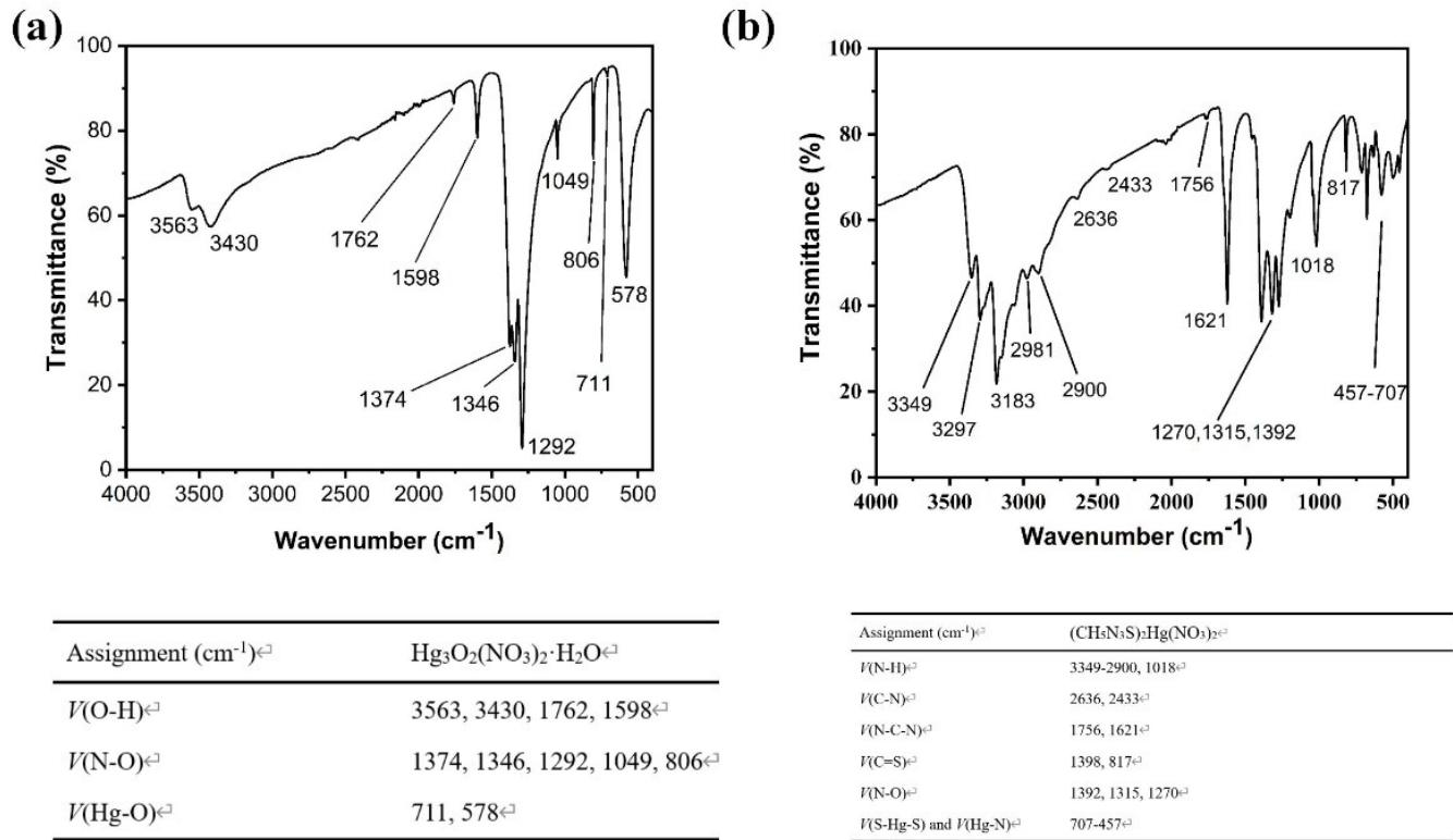
**Figure S5.** IR spectrum and the peaks' assignment for  $\text{Hg}_3\text{O}_2(\text{NO}_3)_2 \cdot \text{H}_2\text{O}$  (a) and  $(\text{CH}_5\text{N}_3\text{S})_2\text{Hg}(\text{NO}_3)_2$  (b).
