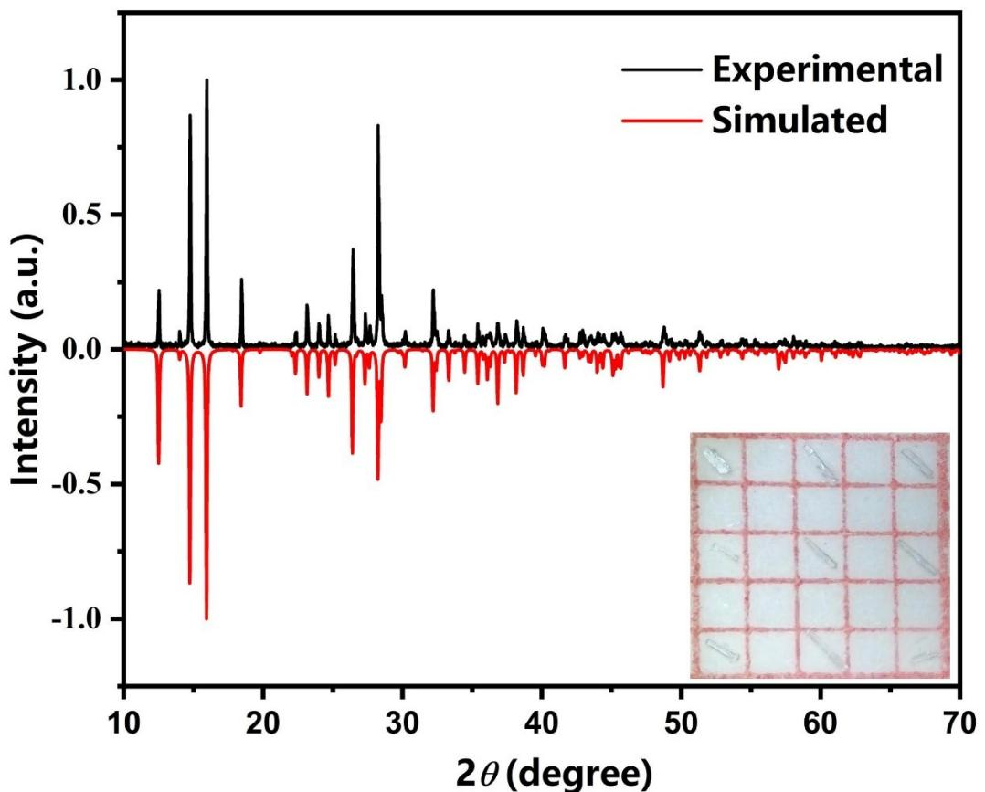
**Figure S2.** Experimental and simulated powder XRD patterns of  $(CH_5N_3S)_2Hg(NO_3)_2$  (1 grid = 1 mm).
