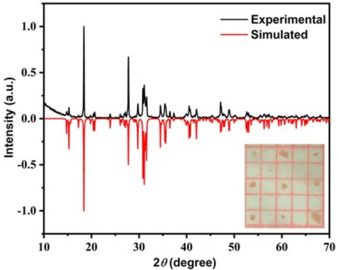
**Figure S1.** Experimental and simulated powder XRD patterns of  $\text{Hg}_3\text{O}_2(\text{NO}_3)_2 \cdot \text{H}_2\text{O}$  (1 grid = 1 mm).
