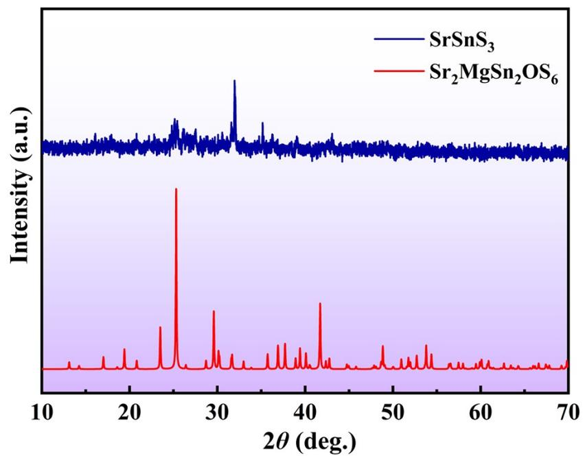
**Figure S3.** Experimental results [(1) blue and (2) purple] and simulated (red) powder XRD patterns of  $\text{Sr}_2\text{MgSn}_2\text{OS}_6$ .
