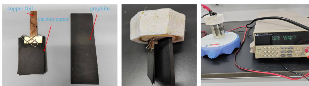
Figure. S3. Reaction setup for the gram scale reaction with batch electrolysis
