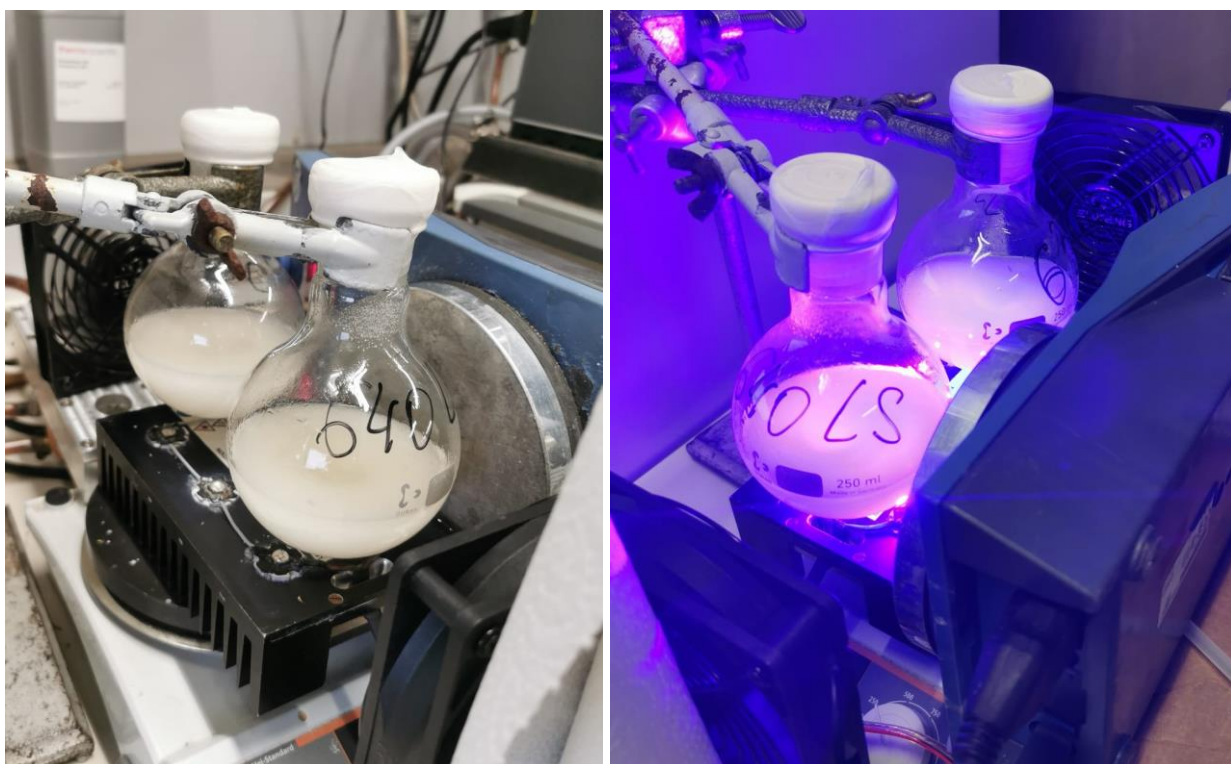
Figure S3. Gram-scale fluorination reactions were conducted by irradiation with LED Engine LZ4-40UB00-00U4 LEDs ( \lambda = 395 nm, 14.8 V, 700 mA).
