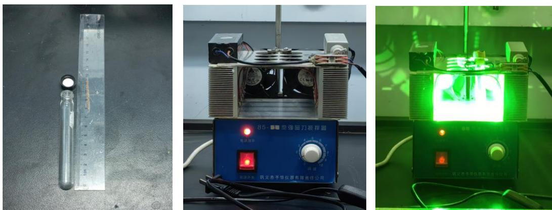
The reaction tube for 0.1 mmol scales (left), green LEDs (5 W  $\times$  8, 505-520 nm) (middle). The reaction tube(s) were irradiated with the green LEDs (right). In each case, the distance between the light source and the reaction vessel was about 2.5 cm.
