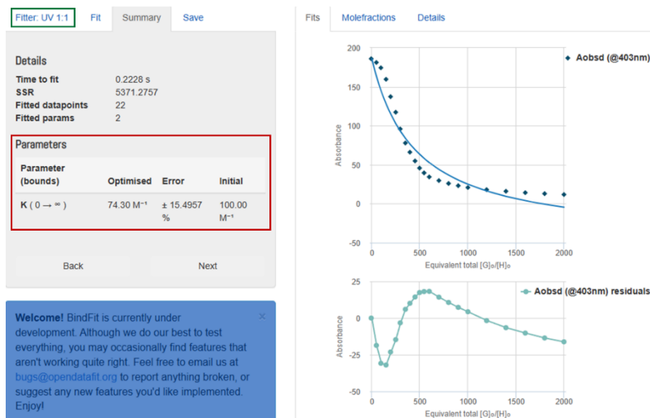
Fig. S2. Screenshot of the summary window of http://app.supramolecular.org/bindfit/ . This screenshot shows the raw data for the fluorescence titration of Py-CT4 with F - with fluorescence emissions at 403 nm vs. the data fitted to a 1:1 UV binding model and the corresponding residual plot and association constants with the calculated asymptotic standard errors.
