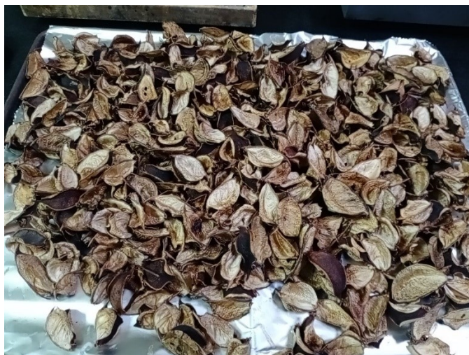
Fig.1: Raw cotton shells after being washed with DI water
