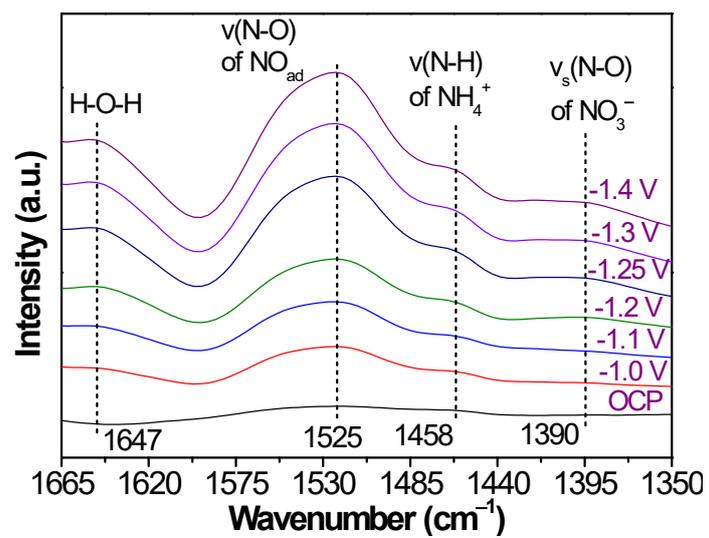
**Fig. S15** *In-situ* ATR-SEIRAS spectra of electrocatalytic NitRR on Cu-Co/BPC at different potentials.
