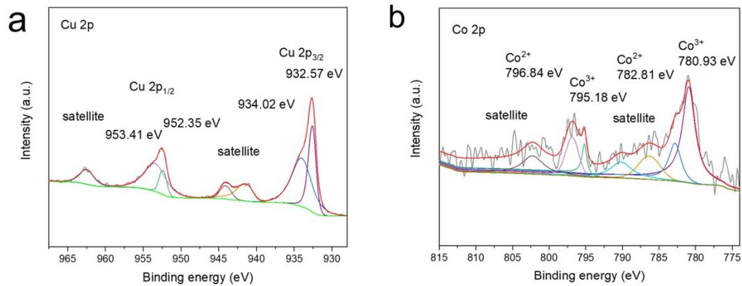
**Fig. S4** High-resolution (a) Cu 2p of Cu/BPC, and (b) Co 2p spectra of Co/BPC
