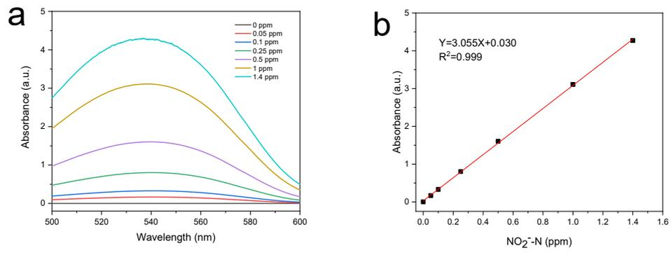
**Fig. S10** (a) UV-Vis absorption spectra obtained from the solutions with different  $\text{NO}_2^-$ -N concentrations (0, 0.05, 0.1, 0.25, 0.5, 1, and 1.4 ppm). (b) Calibration curve used to determine  $\text{NO}_2^-$ -N concentration.
