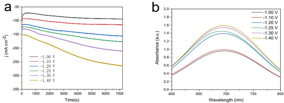
**Fig. S6** (a) Time-dependent current density curves at different potentials in 0.1 M  $\text{N}_2\text{SO}_4$  + 0.1 M N-KNO<sub>3</sub> electrolyte over a 2 h period. (b) UV-Vis absorption spectra obtained from solutions at different potentials.
