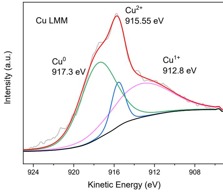
**Fig. S3** Cu LMM XPS spectrum of Cu-Co/BPC.
