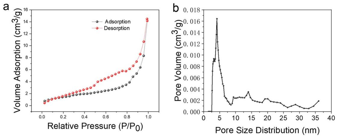
**Fig. S1** (a) Nitrogen adsorption and desorption isotherms of Cu-Co/BPC. (b) Pore size distribution curve of Cu-Co/BPC.
