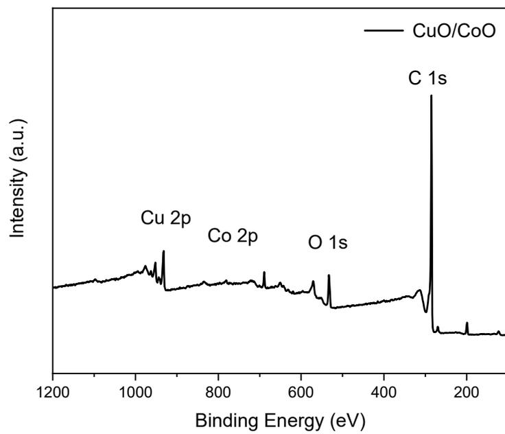
**Fig. S2** Survey XPS spectrum of Cu-Co/BPC.
