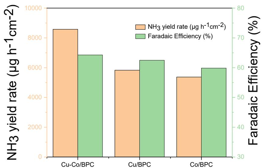
**Fig. S9** Performance comparison of Cu/BPC, Co/BPC and Cu Co/BPC.
