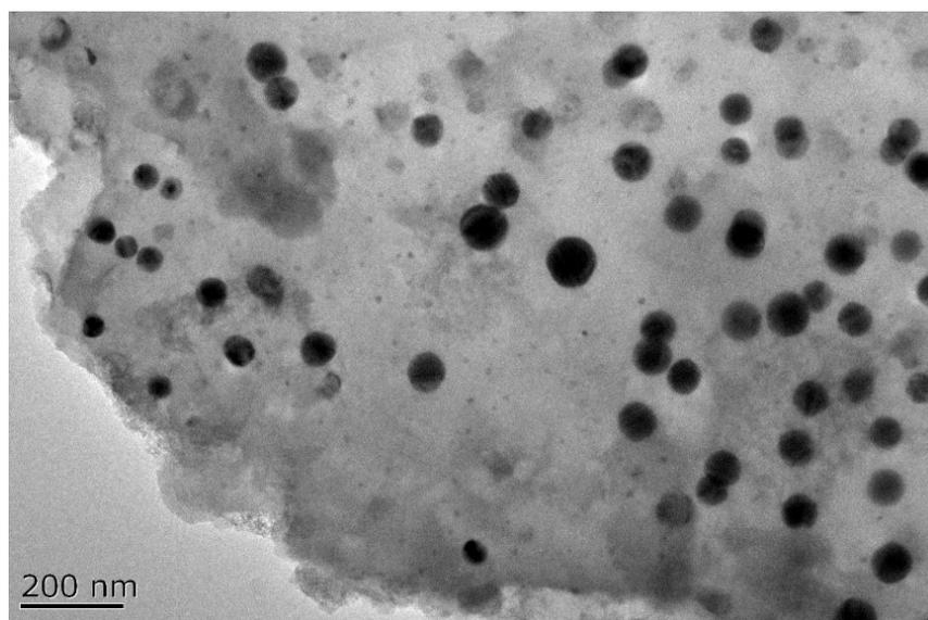
**Fig. S8** The TEM image of Cu-Co/BPC after NitRR.
