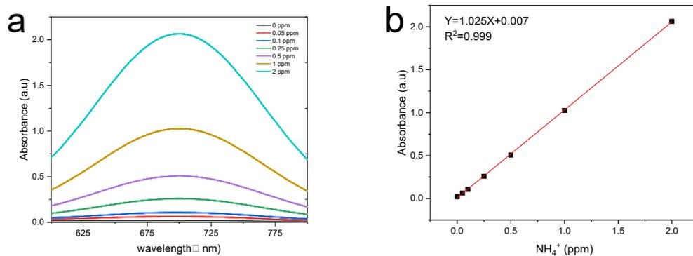
**Fig. S7** (a) UV-Vis absorption spectra of various  $\text{NH}_4^+$ -N concentrations (0, 0.25, 0.50, 0.75, 1, 2 ppm) after incubated for 1 h at room temperature. (b) The calibration curve used for calculation of  $\text{NH}_4^+$ -N concentration.
