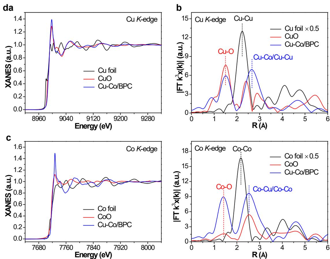
**Fig. S5** Cu *K* edge (a) XANES spectra and (b)  $k^3$ -weighted FT-EXAFS spectra of Cu-Co/BPC and references, Co *K* edge (c) XANES spectra and (d)  $k^3$ -weighted FT-EXAFS spectra of Cu-Co/BPC and references.
