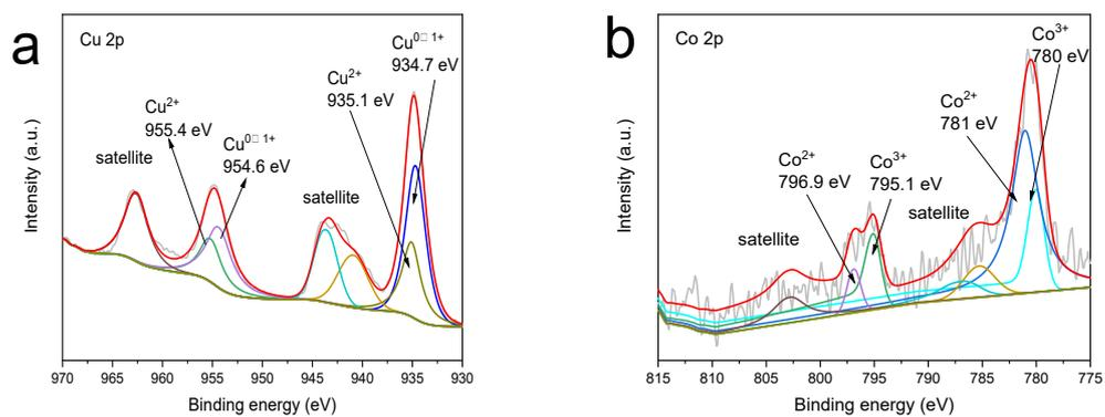
**Fig. S13** High-resolution XPS spectra of (a) Cu 2p, (b) Co 2p of Cu-Co/BPC after NitRR with 6 h.
