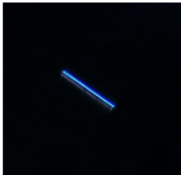
**Figure S3.** Cross Polarized Optical Microscopy image of a  $(\text{BrC}_5\text{H}_{13}\text{N})_3\text{Bi}_2\text{Br}_9$  crystal. The image dimension is  $77 \times 77 \mu\text{m}$ .
