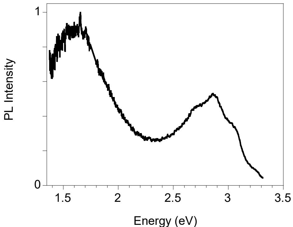
**Figure S4.** Normalized photoluminescence spectrum of a cast film of  $(\text{BrC}_5\text{H}_{13}\text{N})_3\text{Bi}_2\text{Br}_9$  excited at 3.54 eV.
