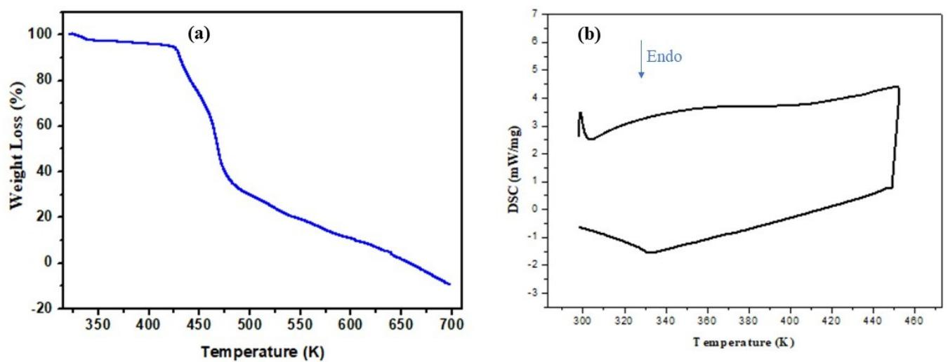
**Figure S2.** (a) The thermogravimetric analysis profile and (b) DSC runs obtained upon heating and cooling for  $(\text{BrC}_5\text{H}_{13}\text{N})_3\text{Bi}_2\text{Br}_9$ .
