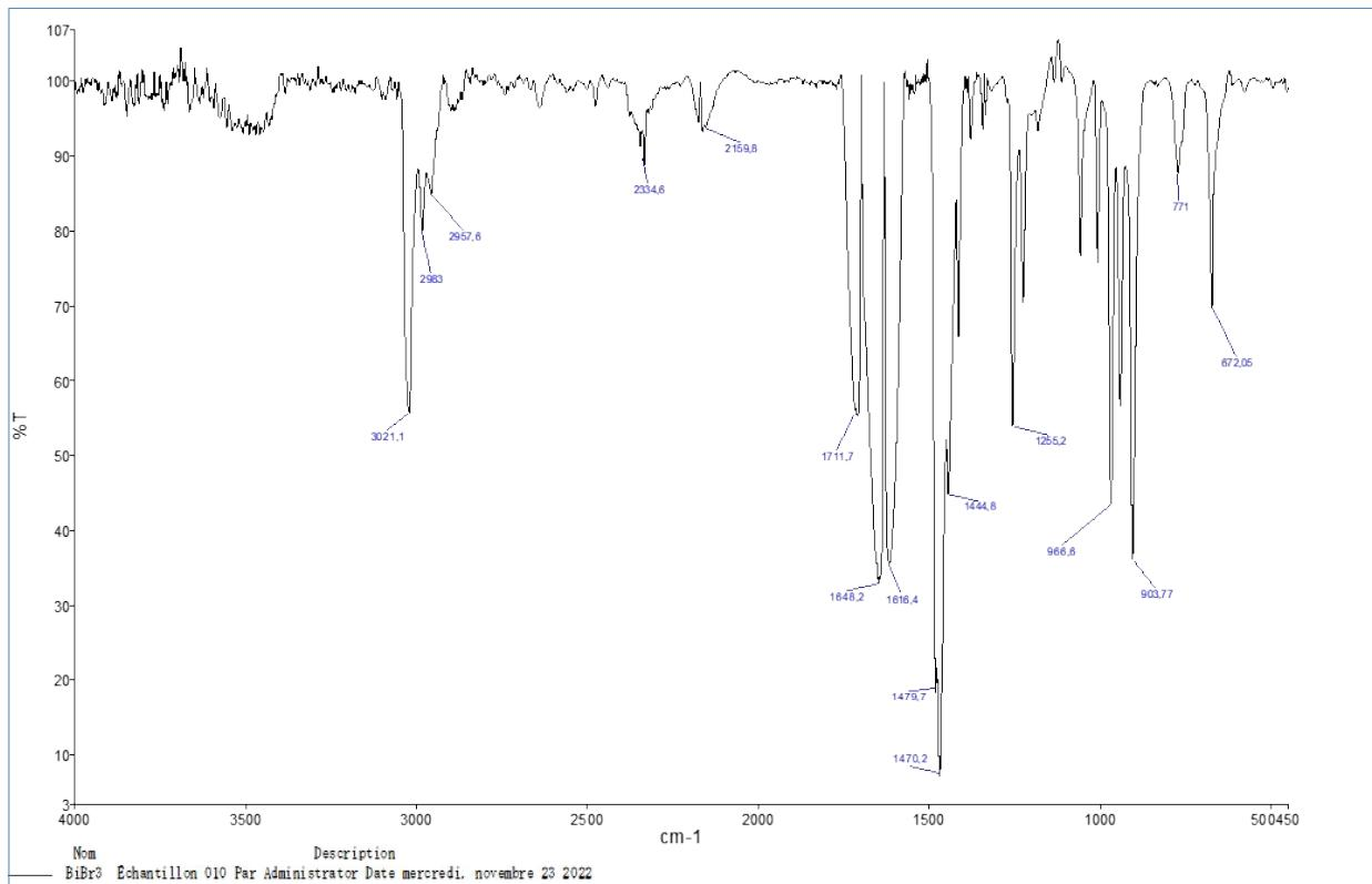
**Figure S1.** IR Spectrum of  $(\text{BrC}_5\text{H}_{13}\text{N})_3\text{Bi}_2\text{Br}_9$ , verifying the phase purity.
